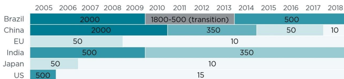
Figure 10 Selected diesel fuel sulfur levels (ppm) in countries and regions around the world. Nationwide standards are shown; Brazil, China, and India have stricter fuel quality in some sub-national and municipal areas (ICCT, 2013)
