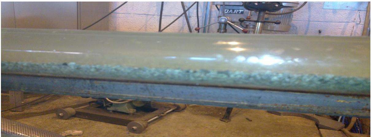
Fig 4.7: Another section of the wellbore, showing the circulation process cuttings.
