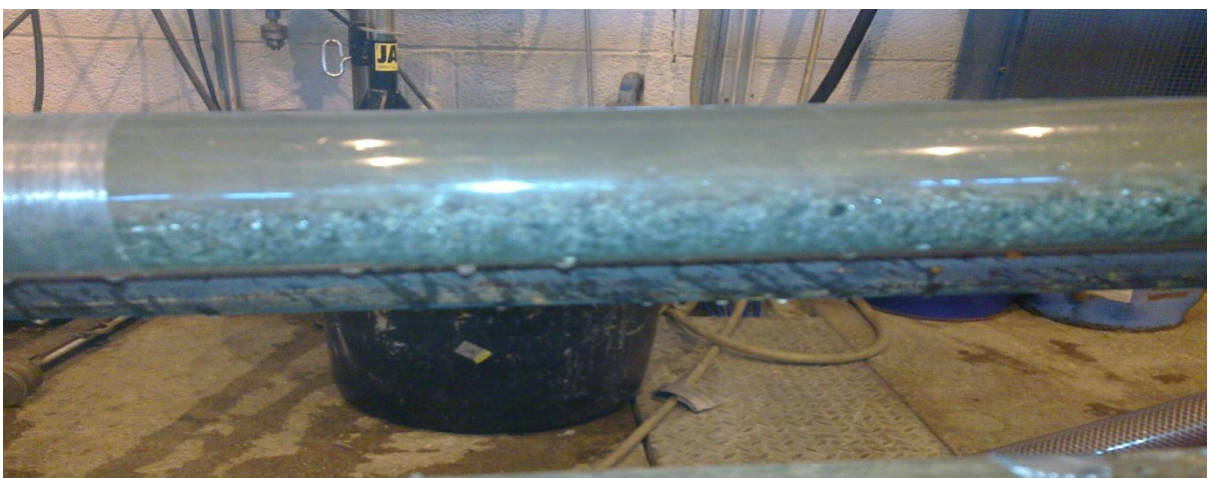
Fig 4.8: Closer look at a cross section of the wellbore, as circulation progresses.
