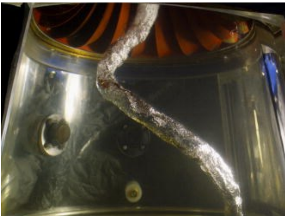
Figure 4 - Vortex rope at part load [24]
