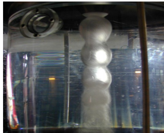
Figure 3 - Vortex rope at high load[24]
