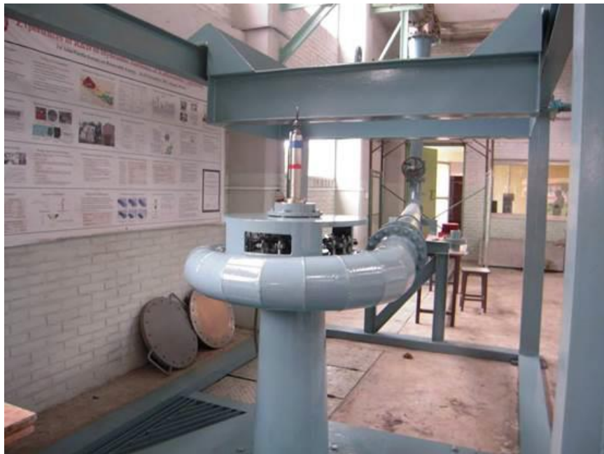
Figure 3.8: Simplified Francis turbine test rig, TTL
