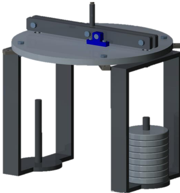
Figure 5.7: 3D representation of the axial force calibration setup.
