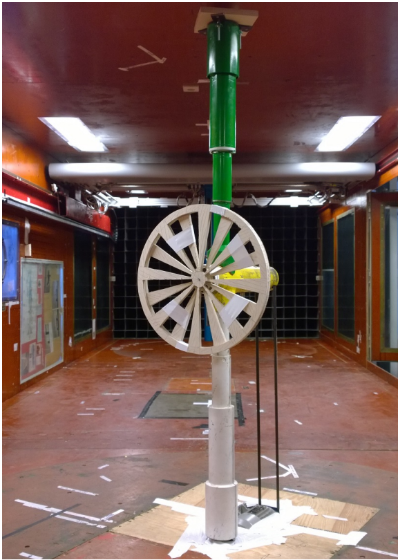
Fig. 3. The disc attached to the turbine with additional tower on top at 30°yaw. Note that the belt was taken off during measurements for symmetry.
