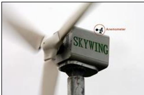
Figure 24. Anemometer in the nacelle.
