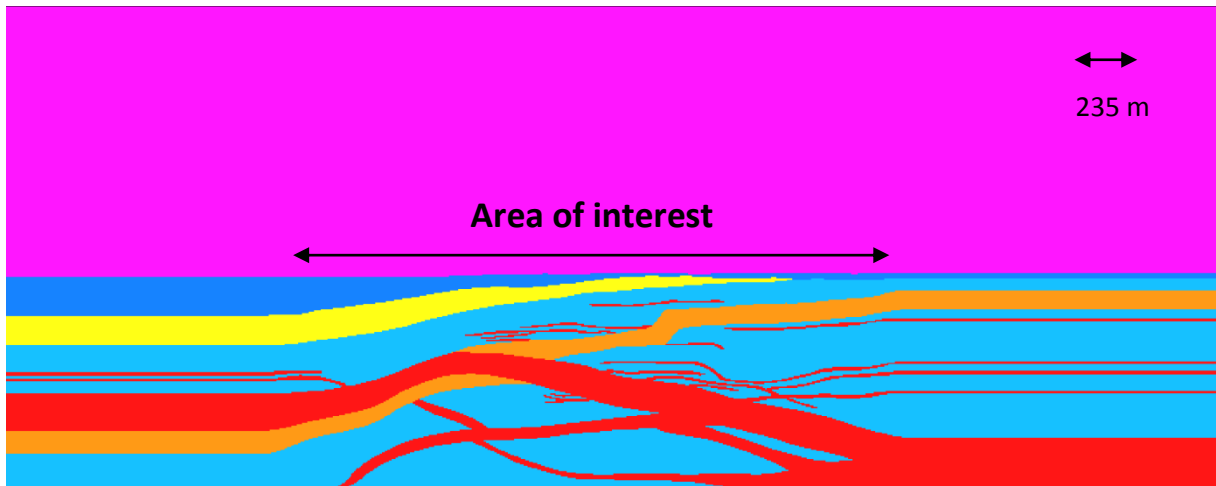
Figure 3.8: Model created in Petrel. The model is extended with 6 km on each side of the actual model (area of interest). The figure above only shows part of the extension.
