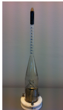
FIGURE B.2: Trial 2, IMBIBITION: artificial core made of 1 mm glass beads and small steel filter. 60 °C in oven. Heavy oil mixture of 30 wt% dodecane and 70 wt% bitumen, and distilled water were used in the trial.
