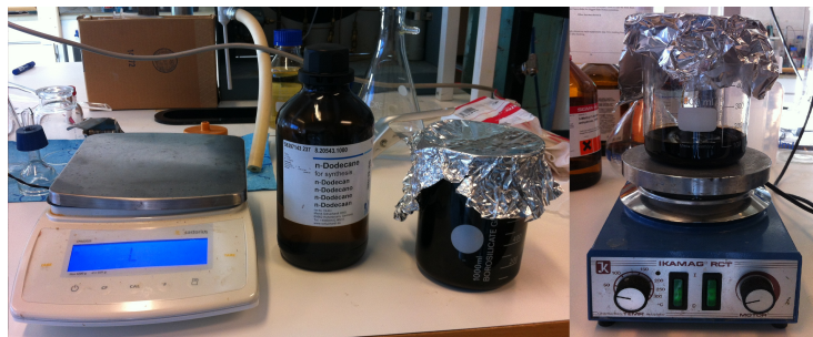
FIGURE 3.2: The equipment needed for mixing of heavy oil. From the left: a weight scale, dodecane and beaker with Athabasca bitumen and a beaker with a stirring magnet on top of the heating/stirring device.
