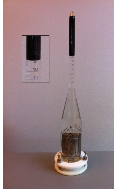
FIGURE B.3: Trial 3, IMBIBITION: artificial core made of 1 mm glass beads and larger steel filter. 60 °C in oven. Heavy oil mixture of 30 wt% dodecane and 70 wt% bitumen, and distilled water were used in the trial.
