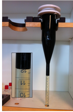
FIGURE B.5: Trial 5, DRAINAGE: artificial core made of 2 mm glass beads. 60 °C in oven. Heavy oil mixture of 30 wt% dodecane and 70 wt% bitumen, and distilled water were used in the trial.
