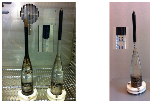
FIGURE D.4: Artificial core made of glass beads soaked in 0.1 wt % hydrophilic nanofluid. From left: Core A, B and C.
