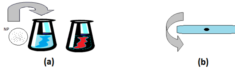
FIGURE 3.15: Schematic drawing of the line of action of the laboratory work that was done for measurement of the interfacial tension. (a) Preparation of fluids. (b) The Spinning drop method.
