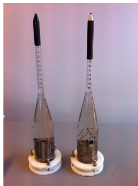
FIGURE B.4: Trial 2 to the right and trial 4 to the left, both are IMBIBITION: see Figure B.2 for details on trial 2. Trial 4: artificial core made of 2 mm glass beads and no filter. 60 °C in oven. Heavy oil mixture of 30 wt% dodecane and 70 wt% bitumen, and distilled water were used in the trial.
