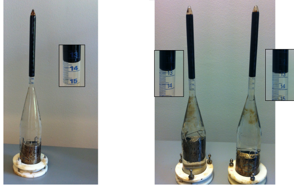
FIGURE D.7: Artificial core made of glass beads soaked in 0.1 wt % hydrophobic nanofluid. The picture is of Core B. No pictures was taken for Core A and Core C. Core A was aborted due to improper cleaning of Amott cell. For Core C no oil came out. Core was left saturated in heavy oil for 2 days.
