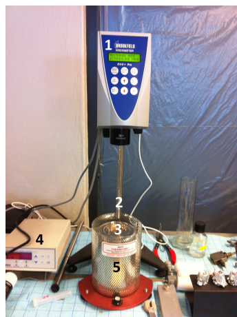
FIGURE 3.5: Setup of the rotating viscometer. 1: the main part of the rotometer. 2: the needle. 3: where the small cylinder with heavy oil is placed. 4: controlling panel for the temperature of the thermosel. 5: the thermosel.
