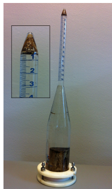
FIGURE B.8: Trial 9, IMBIBITION: artificial core made of 425 – 600 \mu\text{m} glass beads and small steel filter. 60 °C in oven. Heavy oil mixture of 30 wt% dodecane and 70 wt% bitumen, and distilled water were used in the trial. Core was left in vacuum pump for two hours in oven before it was put into the Amott cell.
