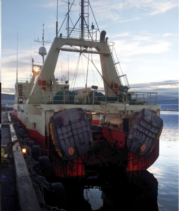
Picture 26 (top): Bottom trawl net with bobbins Picture 27 (bottom left): Bottom trawl doors. Picture 28 (bottom right): The same bottom trawl doors on a trawler, as one can see the doors are large.
