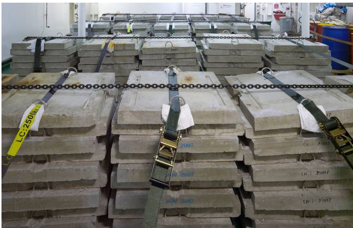
Picture 39: The concrete anchors EMGS use for their seabed receivers are more or less just square slabs of concrete.
