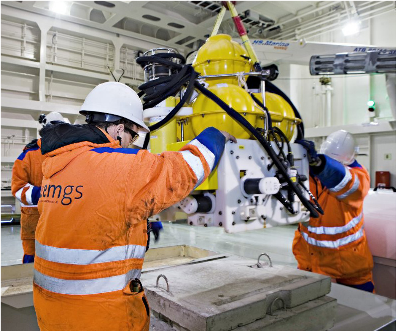
Picture 2: Workers at EMGS assembling a data logging receiver, the water soluble concrete anchor can here be seen.
