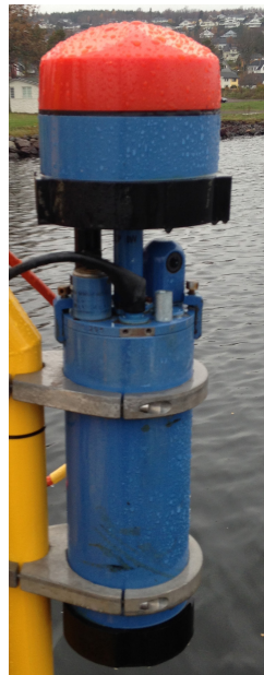
SEAGUARD Recording Current Meter (ACDP) Diameter: 140 mm Length: 352 mm Weight in air: 11.5 kg, in water: 5.2 kg
