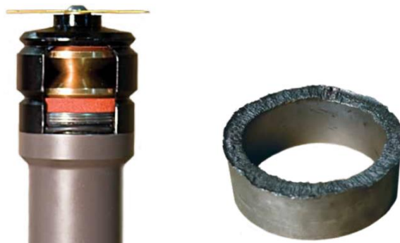
Figure 5-20: Explosive Cutting tool and a pipe end after cutting with an explosive cutting tool [44].
