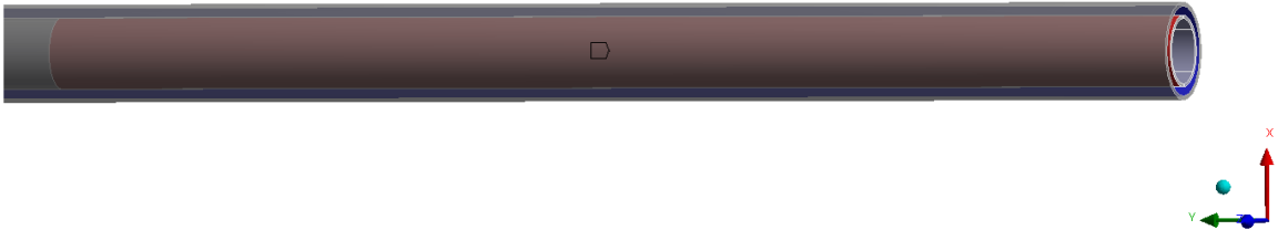
Figure 5-9: Contact setup between the tubing and casing.
