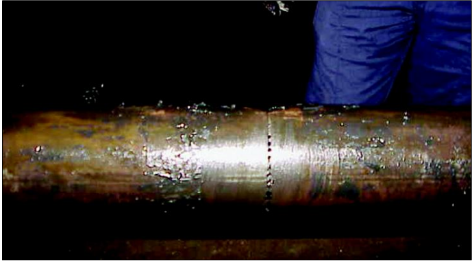
Figure 5-19: Cut performed by a chemical cutter [43].
