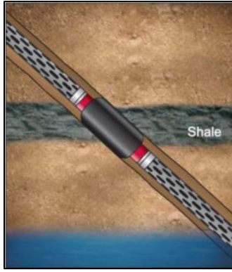
Figure 5-22: Inflatable packer used for zonal isolation [52].
