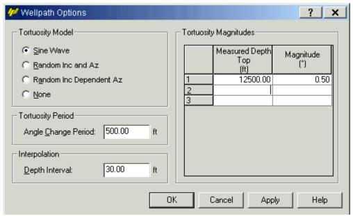
Figure 137: Well path tortuosity input for the drilling of 9 1/2" section from junction to TD for MLT1 Lateral 1 (Wellplan 2013)
