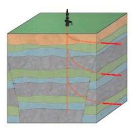
Figure 71: Reservoir with separated reservoir compartments penetrated by a multilateral well with three branches (Frailia et al. 2002)
