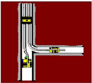
Figure 14: TAML Level 5 Junction (Weatherford 2006)
