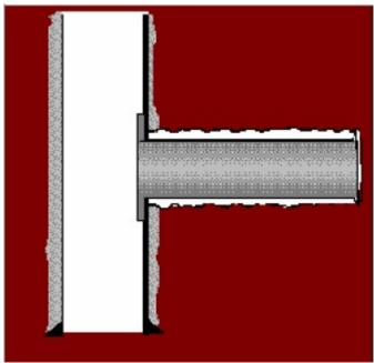
Figure 12: TAML Level 3 Junction (Weatherford 2006)
