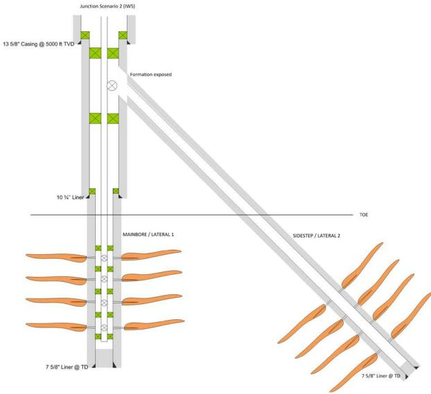
Figure 20: Junction design option 2 installed and ready for production. The figure is not scaled, nor are the proper inclinations shown. Should be used for information purposes only (Figure made by this author)
