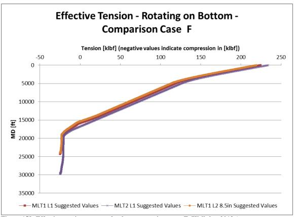
Figure 158: Effective tension suggested values comparison case F (Wellplan 2013a)
