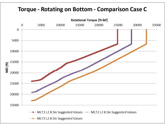
Figure 165: Torque suggested values comparison case C (Wellplan 2013a)
