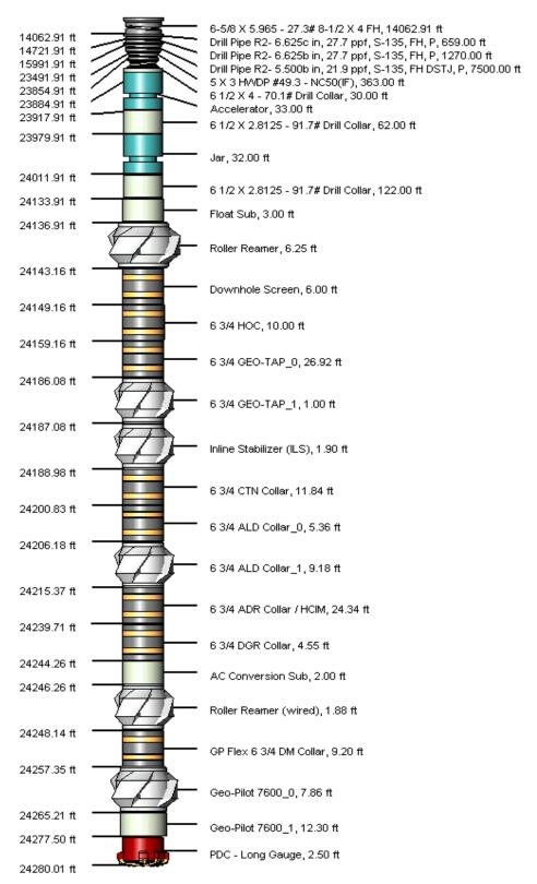
Figure 134: Initial BHA schematic for the drilling of the 9 ½" hole section from junction to TD for MLT1 Lateral 1 (Wellplan 2013a)
