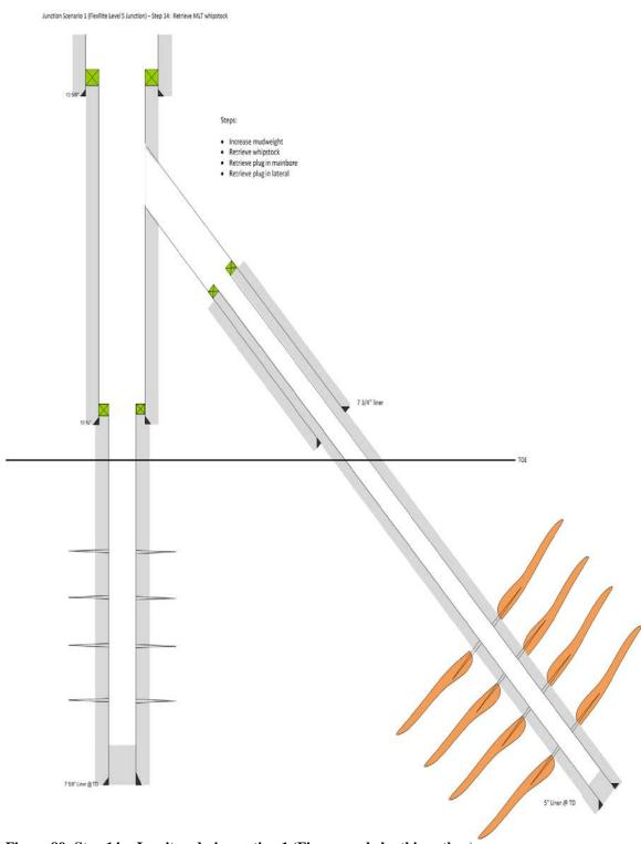
Figure 89: Step 14 – Junciton design option 1 (Figure made by this author)
