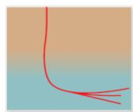
Figure 75: Example of a forked ML (Bosworth et al. 1996)
