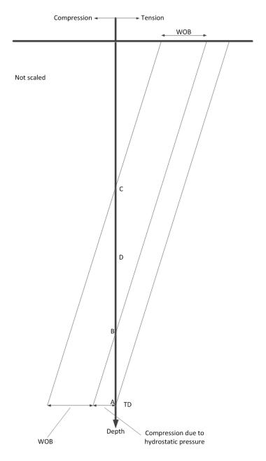
Figure 30: Effect of buoyancy on buckling in form of neutral point of tension and NPB (Figure made by this author)
