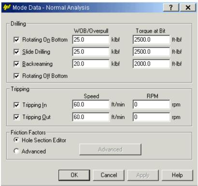
Figure 149: Torque and Drag Setup with WOB, torque at bit and tripping speed for Scenario 2 (Wellplan 2013)
