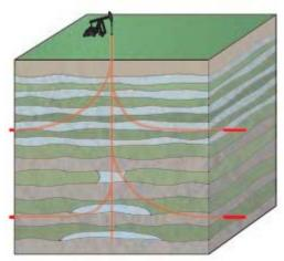
Figure 70: MLT applied in a laminated, or layered, formation (Frailja et al. 2002)
