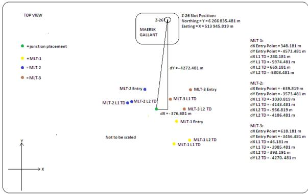
Figure 23: Top view of the MLT set-up for well slot 2/4-Z-26 with junction placement and the three multilateral configurations s to be investigated. All positions and differential distances are with regards to the slot coordinates (Figure made by this author)
