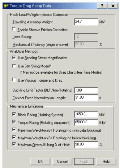
Figure 144: Torque and Drag Setup Data used for both Scenario 1 and Scenario 2 (Wellplan 2013a)
