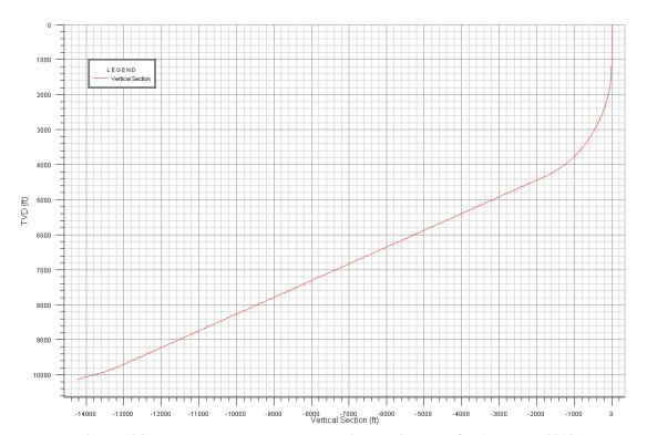
Figure 104: Mother wellbore well path vertical sections to TOE (Wellplan 2013a)
