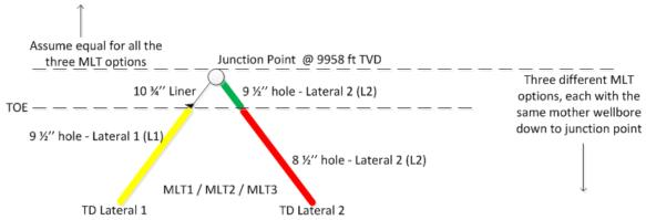
Figure 37: Hole sizes to be drilled for all of the three MLT options for junction design option 2, with IWS. Same as Figure 21 (Figure made by this author)
