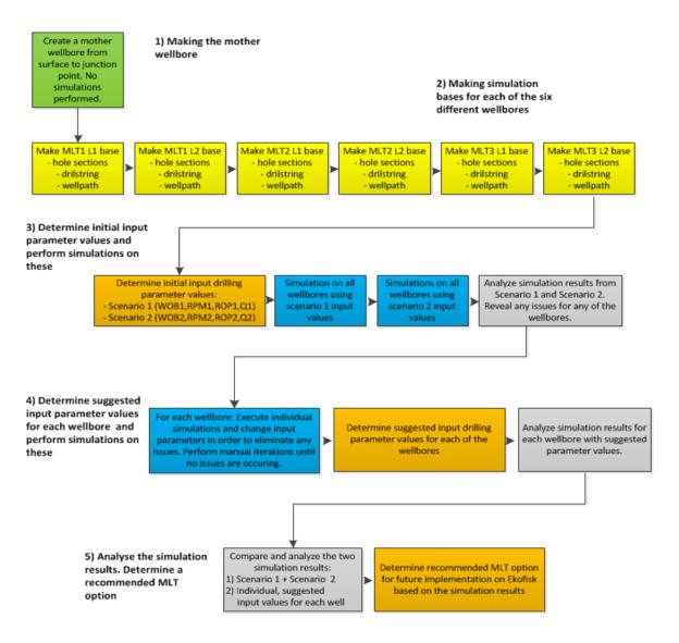
Figure 32: Step-wise process of the simulations performed in Wellplan (Figure made by this author)
