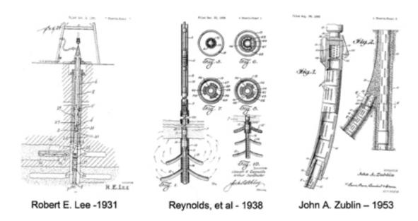
Figure 66: Technical drawings of the first patents on multilateral well technology (E&P Magazine 2007)
