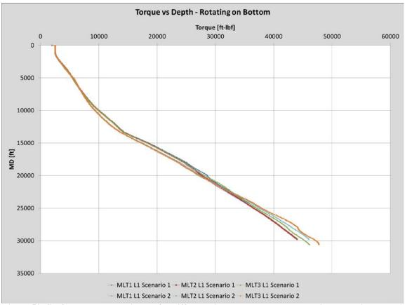
Figure 50: Surface torque experienced for different bit depths as each wellbore in comparison case A is drilled to TD with scenario 1 and 2 input parameter values (Wellplan 2013)
