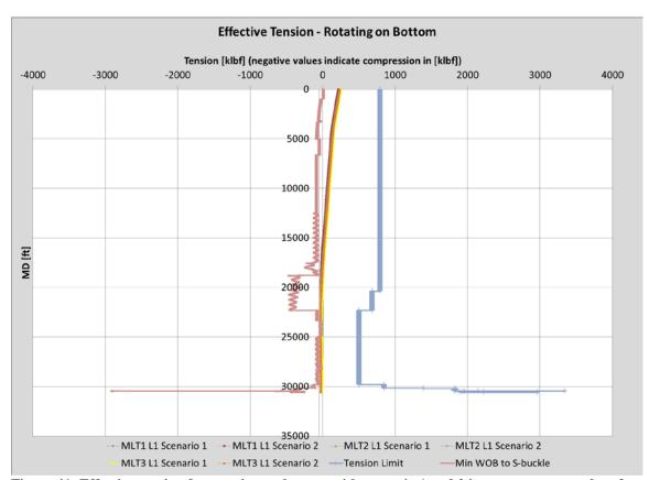
Figure 41: Effective tension for rotating on bottom with scenario 1 and 2 input parameter values for comparison case A. Left red line indicates minimum WOB to sinusoidal buckle the drillstring, while the right blue line displays the tension limit/tensile strength for the drillstring components at different measured depths (Wellplan 2013a)
