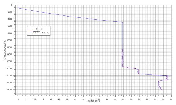
Figure 138: Well path inclination with tortuosity for the drilling of the  $9\frac{1}{2}$ " section from junction to TD for MLT1 Lateral 1 (Wellplan 2013)
