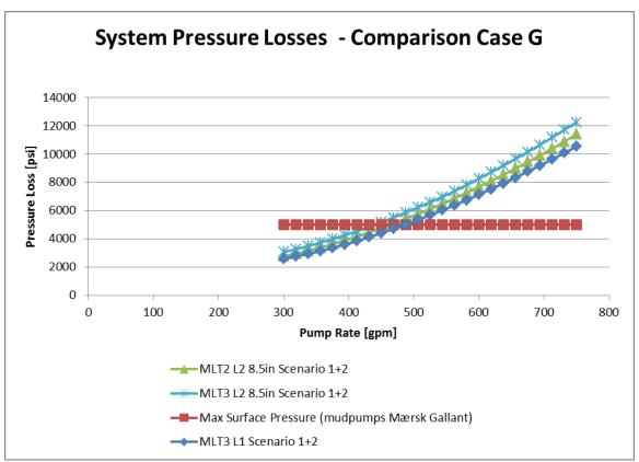
Figure 187: Pressure losses scenario 1 and 2 values comparison case G (Wellplan 2013a)
