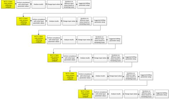
Figure 33: Schematic of the step-wise iteration process for each of the wellbores in order to find the individual, suggested drilling parameter values (Figure made by this author)
