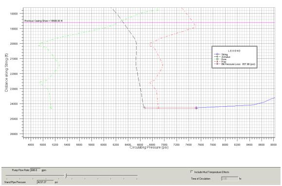
Figure 60: Circulating pressure for MLT1 L1 for suggested parameter input values (Wellplan 2013a)
