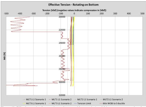
Figure 42: Effective tension for rotating on bottom with scenario 1 and 2 input parameter values for comparison case A. The left red line indicates minimum WOB to sinusoidal buckle the drillstring. As long as the effective tension values are to the right-hand side of the minimum WOB sinusoidal buckling will not occur (Wellplan 2013a)
