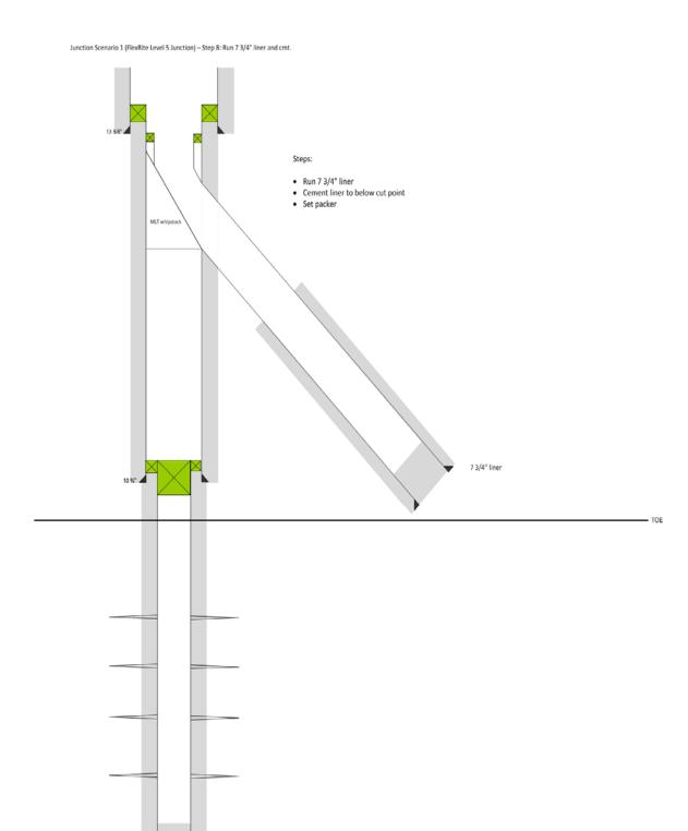
Figure 86: Step 8 – Junciton design option 1 (Figure made by this author)
