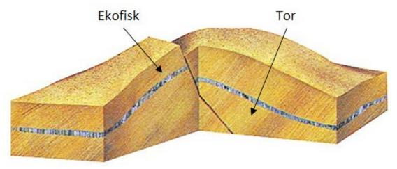
Figure 2: Illustration of the Ekofisk reservoir, with Ekofisk and Tor formation (ConocoPhillips 2013f)
