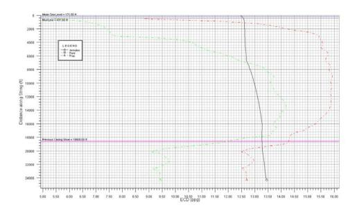
Figure 62: ECD vs MD for MLT1 L1 scenario 2 input values (Wellplan 2013a)
