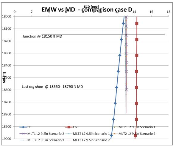
Figure 193: ECD for scenario 1 and 2 values comparison case D (Wellplan 2013a)
