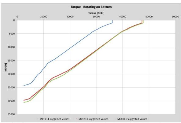
Figure 45: Rotary torque in the drillstring for bit rotating on bottom for the suggested input parameter values for comparison case A (Wellplan 2013a)
