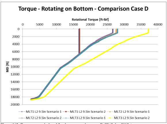
Figure 162: Torque scenario 1 and 2 values comparison case D (Wellplan 2013a)
