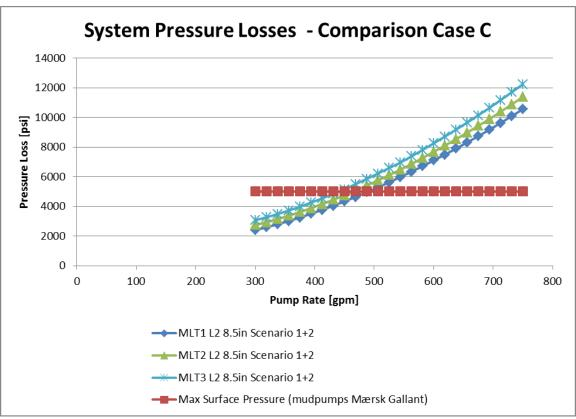
Figure 184: Pressure losses scenario 1 and 2 values comparison case C (Wellplan 2013a)
