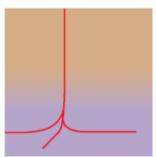
Figure 78: 3D example of a chicken foot, or multibranched, multilateral well (Bosworth et al. 1996)
