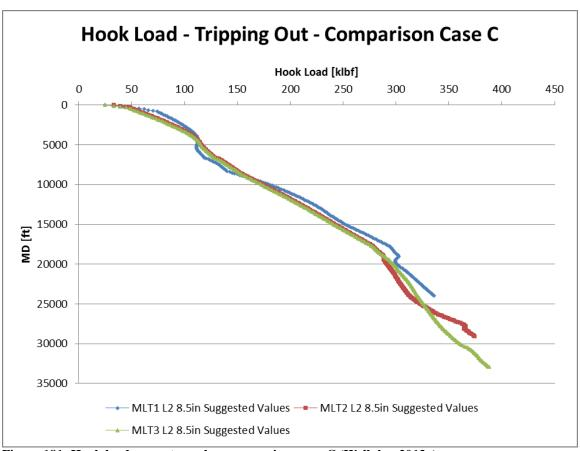
Figure 181: Hook load suggestev values comparison case C (Wellplan 2013a)
