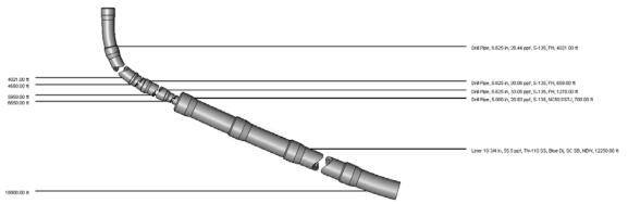
Figure 130: Component schematic for the running of  $10\,\%$ " liner in mainbore (to scale) (Wellplan 2013a)
