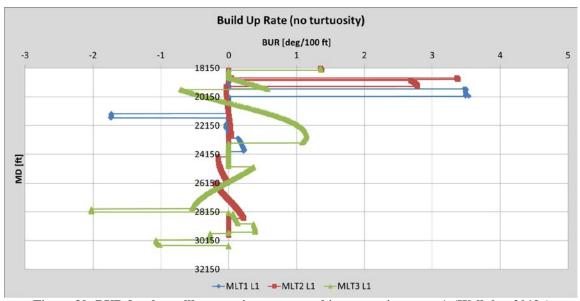
Figure 39: BUR for the wellbore sections compared in comparison case A (Wellplan 2013a)
