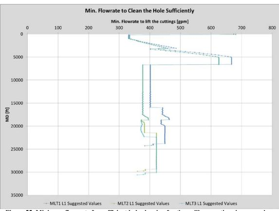
Figure 55: Minimum flow rate for sufficient hole cleaning for the wellbore sections in comparison case A with suggested parameter values (Wellplan 2013a)
