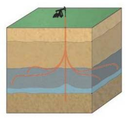
Figure 73: MLT applied in a heavy oil deposit, either as producer or steam injector (Frailja et al. 2002)
