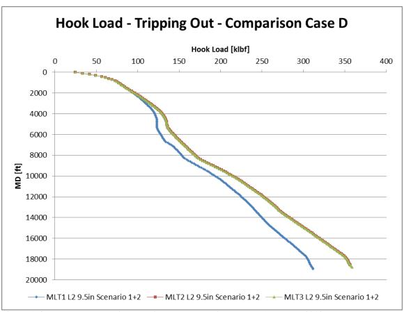
Figure 178: Hook load scenario 1 and 2 values comparison case D (Wellplan 2013a)
