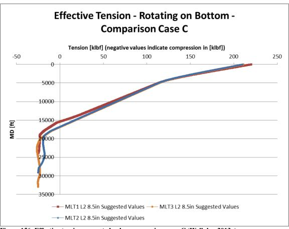
Figure 156: Effective tension suggested values comparison case C (Wellplan 2013a)
