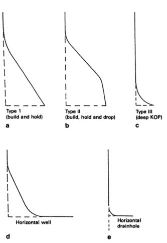
Figure 25: Examples of build-up, hold and drop for deviated and horizontal wells (Inglis 1987)
