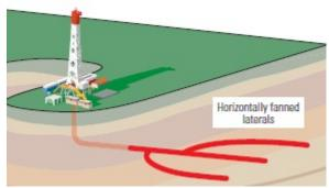
Figure 68: Horizontally fanned laterals can reduce friction pressure drop compared to a single, long horizontal wellbore section (Frailia et al. 2002)
