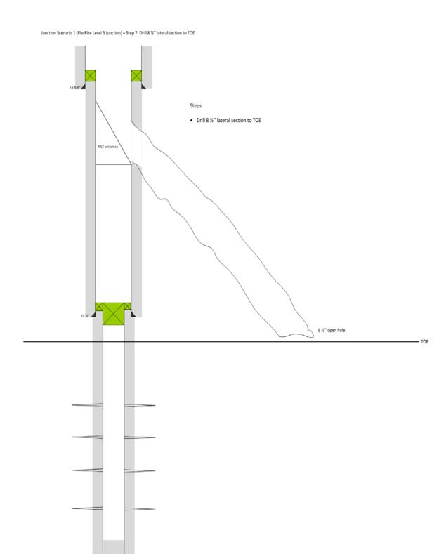
Figure 85: Step 7 – Junciton design option 1 (Figure made by this author)
