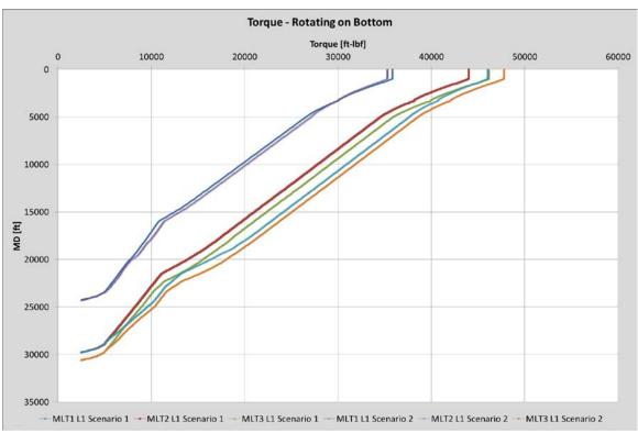
Figure 44: Rotary torque in the drillstring for bit rotating on bottom for scenario 1 and 2 input parameter values for comparison case A (Wellplan 2013a)
