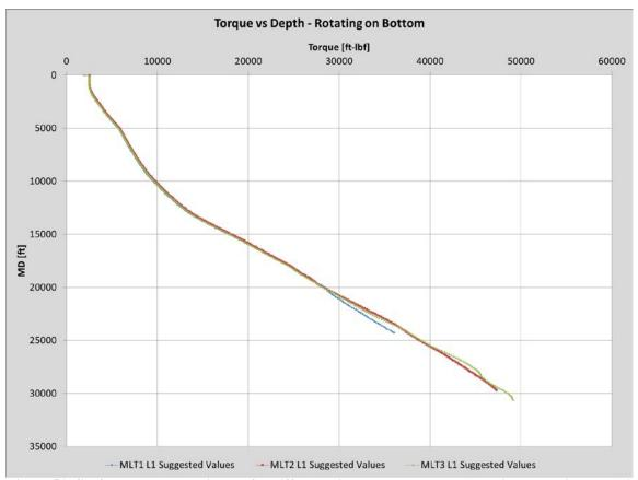
Figure 51: Surface torque experienced for different bit depths as each wellbore in comparison case A is drilled to TD with suggested parameter values (Wellplan 2013)
