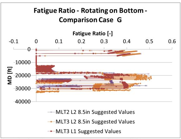
Figure 176: Fatigue ratio suggested values comparison case G (Wellplan 2013a)
