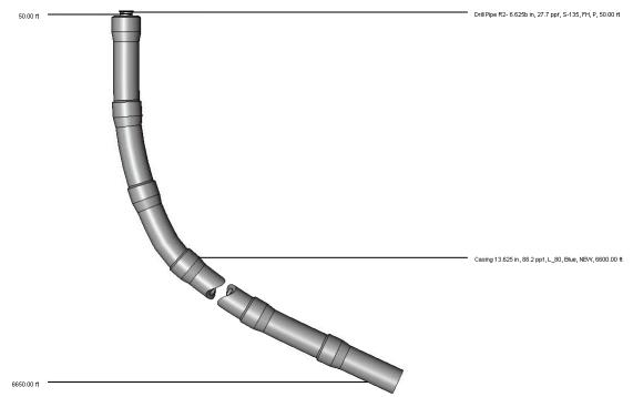
Figure 122: Component schematic for the running of 13 5/8" casing in mainbore (to scale) (Wellplan 2013a)
