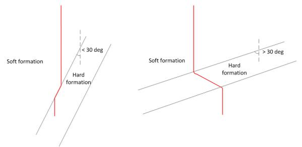
Figure 24: High DLS caused by the entering of a harder formation at inclination (Figure made by this author)
