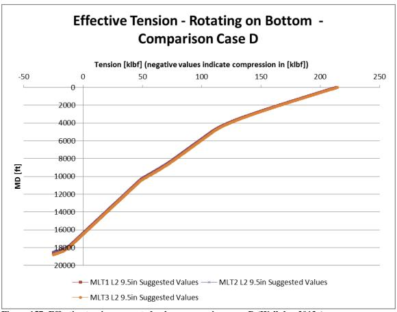
Figure 157: Effective tension suggested values comparison case D (Wellplan 2013a)
