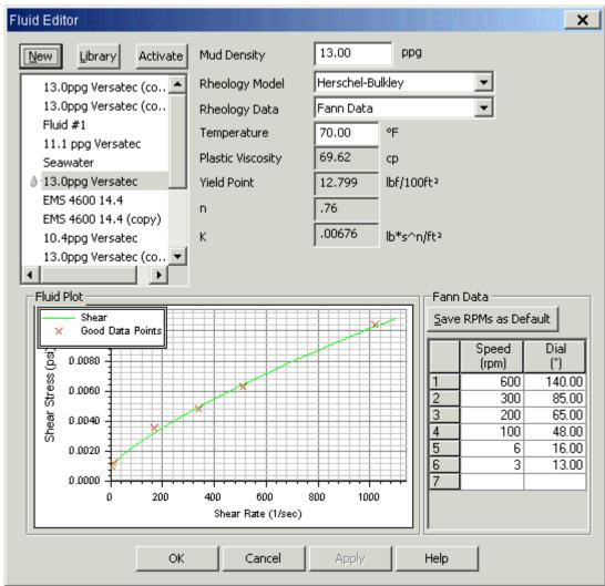
Figure 119: Mud program for the drilling of the 16" hole section in mainbore (Wellplan 2013a)
