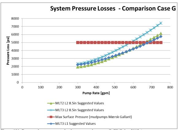
Figure 191: Pressure losses suggested values comparison case G (Wellplan 2013a)
