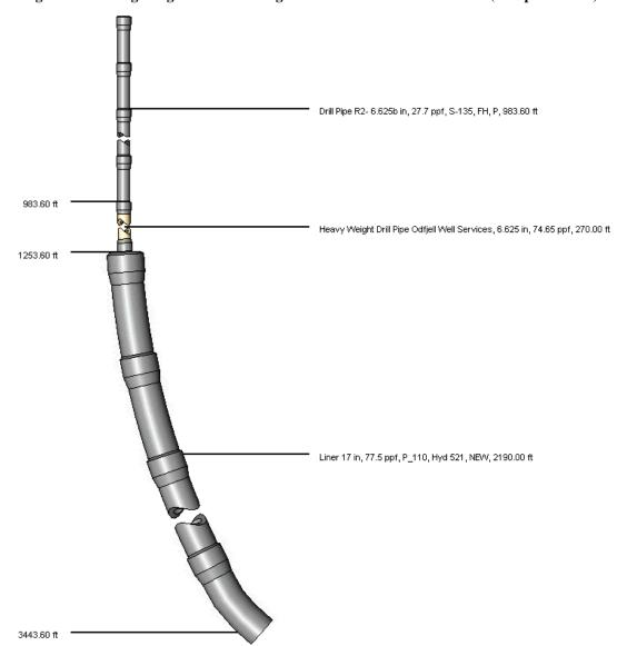
Figure 114: Component schematic for the running of 17" liner in mainbore (to scale) (Wellplan 2013a)
