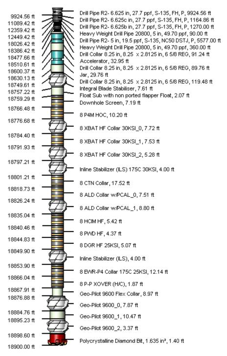
Figure 126: BHA Schematic for the drilling of  $12\,\%$  hole section in mainbore (non-deviated, not to scale) (Wellplan 2013a)
