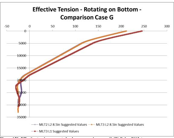
Figure 159: Effective tension suggested values comparison case G (Wellplan 2013a)
