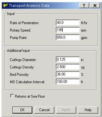
Figure 150: Transport analysis data initial setup for Scenario 2 (Wellplan 2013)
