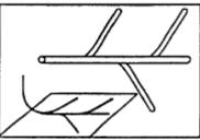
Figure 80: Example of a planar opposed multilateral well, 3D and top view (Crouse 1996)
