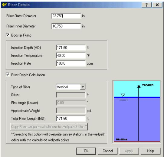
Figure 106: Riser booster pump configuration for both Scenario 1 and Scenario 2 (Wellplan 2013)
