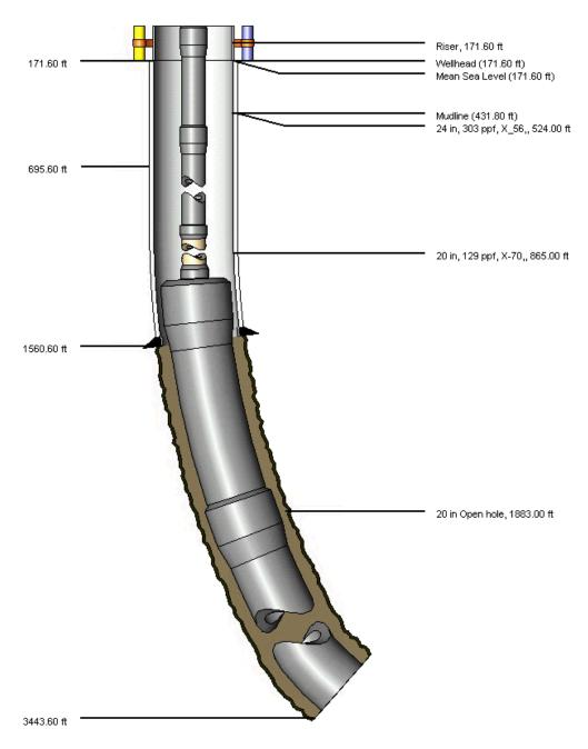
Figure 112: Schematic of hole sections with string for running of the 17" liner in mainbore (to scale) (Wellplan 2013a)
