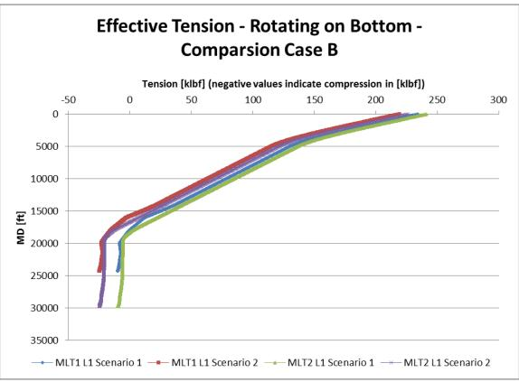
Figure 151: Effective tension scenario 1 and 2 comparison case B (Wellplan 2013a)
