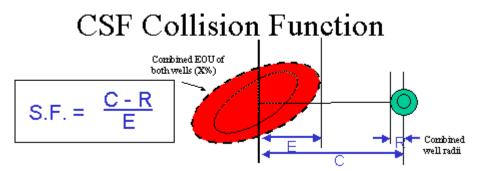
Figure 101: Separation Factor (SF) (Compass 2013b)
