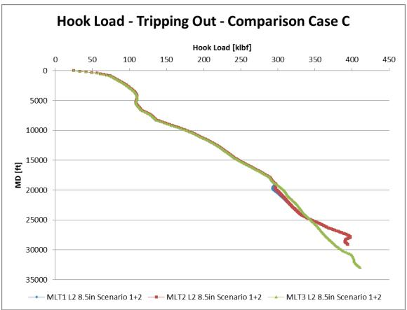
Figure 177: Hook load scenario 1 and 2 values comparison case C (Wellplan 2013a)
