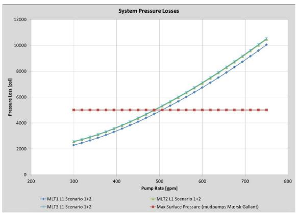
Figure 56: System pressure losses for wellbores in comparison case A with scenario 1 and scenario 2 parameter input values (Wellplan 2013a)
