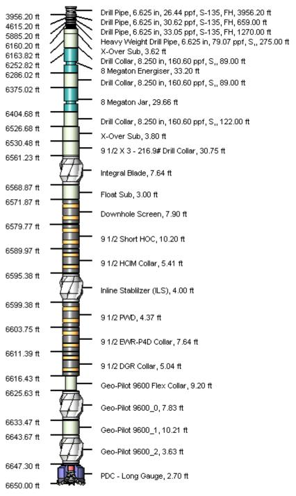
Figure 118: BHA Schematic for the drilling of 16" hole section in mainbore (non-deviated, not to scale) (Wellplan 2013a)
