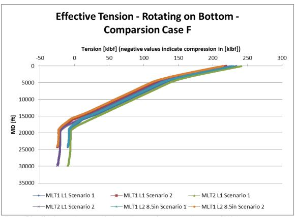
Figure 154: Effective tension scenario 1 and 2 comparison case F (Wellplan 2013a)
