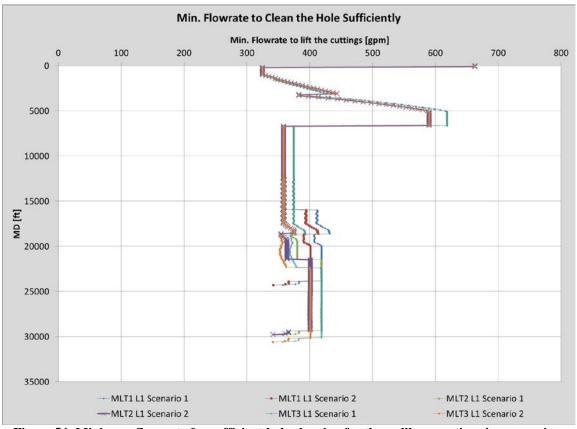
Figure 54: Minimum flow rate for sufficient hole cleaning for the wellbore sections in comparison case A with scenario 1 and 2 input parameter values (Wellplan 2013a)
