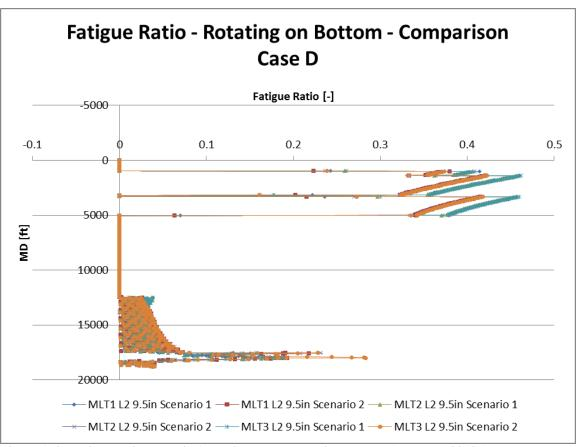
Figure 170: Fatigue ratio scenario 1 and 2 values comparison case D (Wellplan 2013a)
