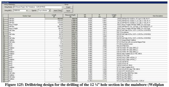
Figure 125: Drillstring design for the drilling of the 12 1/4" hole section in the mainbore (Wellplan 2013a)
