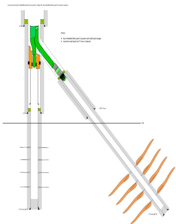
Figure 91: Step 16 – Junciton design option 1 (Figure made by this author)
