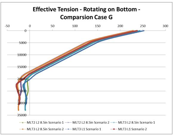
Figure 155: Effective tension scenario 1 and 2 comparison case G (Wellplan 2013a)
