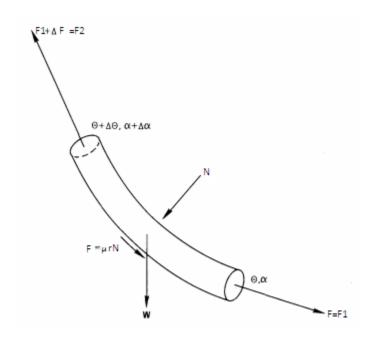
Figure 27: Forces on a pipe section element for torque and drag analysis using the discrete model (Johancsik et al. 1984)
