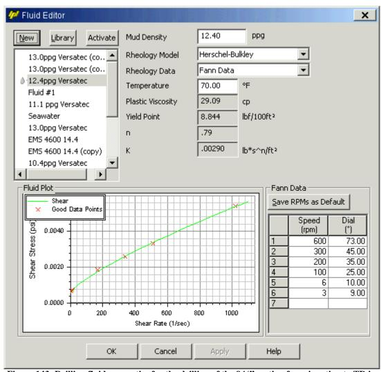
Figure 143: Drilling fluid properties for the drilling of the  $9\,1\!/2$ ' section from junction to TD in Ekofisk for MLT1 Lateral 1 (Wellpan 2013)
