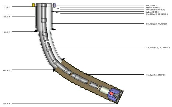
Figure 115: Schematic of hole sections with drillstring for the 16" drilling in mainbore (to scale) (Wellplan 2013a)
