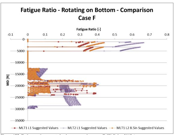
Figure 175: Fatigue ratio suggested values comparison case F (Wellplan 2013a)
