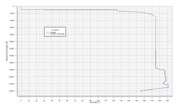
Figure 139: Well path azimuth with tortuosity for the drilling of the  $9\frac{1}{2}$  section from junction to TD for MLT1 Lateral 1 (Wellplan 2013)
