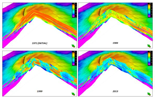
Figure 3: Reservoir model of oil saturation in Ekofisk as a function of time (ConocoPhillips 2013h)
