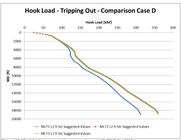
Figure 182: Hook load suggestev values comparison case D (Wellplan 2013a)
