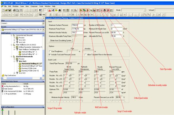
Figure 141: Overview of the different modules in Wellplan (Wellplan 2012)
