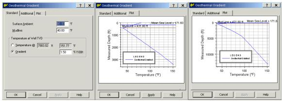
Figure 105: Geothermal gradient input in Wellplan for the mainbore (Wellplan 2013a)
