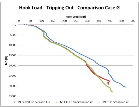
Figure 180: Hook load scenario 1 and 2 values comparison case G (Wellplan 2013a)
