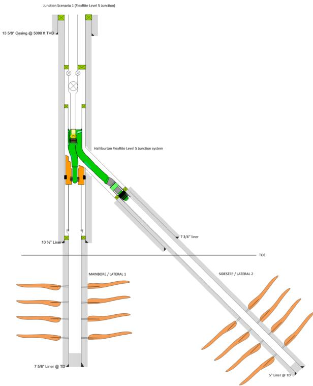
Figure 19: Junction design option 1 installed and ready for production. The figure is not scaled, nor are the proper inclinations shown. Should be used for information purposes only (Figure made by this author)
