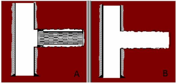
Figure 11: TAML Level 2A and Level 2B Junctions (Weatherford 2006)
