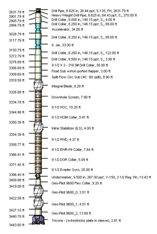
Figure 110: BHA Schematic for the drilling of 20" x 17 ½" hole section in mainbore (non-deviated, not to scale) (Wellplan 2013a)
