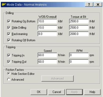
Figure 147: Torque and Drag Setup with WOB, torque at bit and tripping speed for Scenario 1 (Wellplan 2013)
