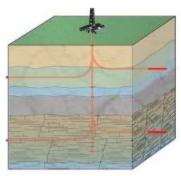
Figure 69: MLT applied in a natural fractured reservoir (Frailja et al. 2002).
