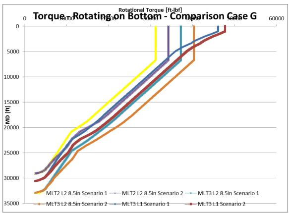
Figure 164: Torque scenario 1 and 2 values comparison case G (Wellplan 2013a)
