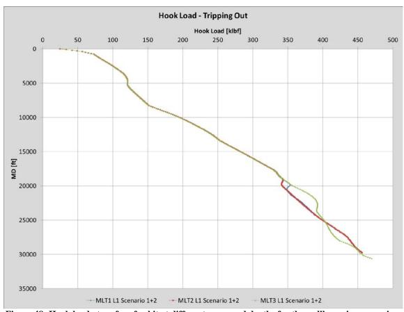
Figure 48: Hook load at surface for bit at different measured depths for the wellbores in comparison case A with scenario 1 and 2 input values (Wellplan 2013a)
