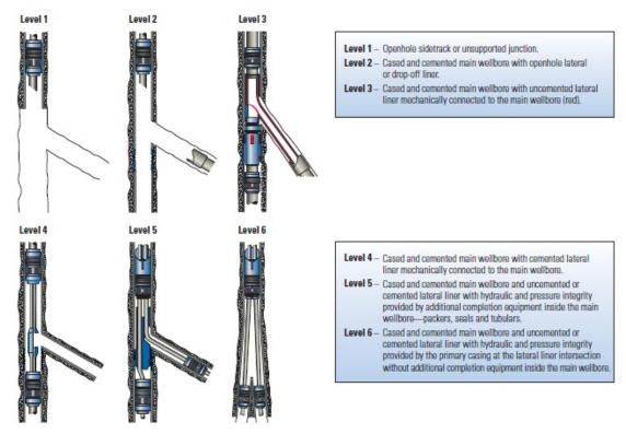
Figure 9: TAML junction classification for Multilateral Wells (Frailja, J., Ohmer, H. and Pulick, T. et al. 2002).
