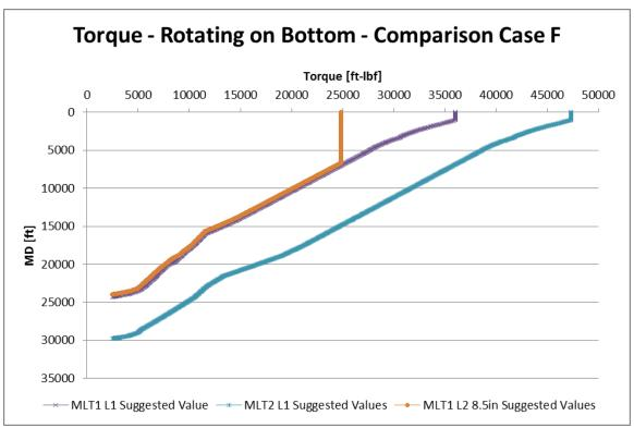
Figure 167: Torque suggested values comparison case F (Wellplan 2013a)
