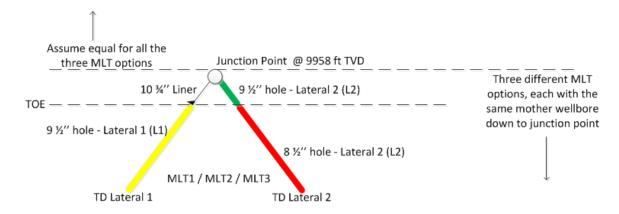
Figure 21: Hole sizes to be drilled for all of the three MLT options for junction design option 2, with IWS (Figure made by this author)
