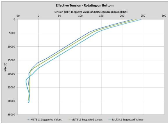
Figure 43: Effective tension for rotating on bottom with suggested input parameter values for comparison case A (Wellplan 2013a)
