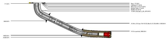
Figure 133: Well schematic for the drilling of the 9  $\frac{1}{2}$ " hole section from junction to TD for MLT1 Lateral 1 (Wellplan 2013a)
