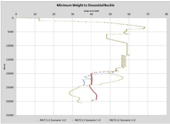
Figure 52: Minimum WOB to sinusoidal buckle for the wellbore sections gathered in the comparison case A for scenario 1 and scenario 2 input parameter values (Wellplan 2013a)
