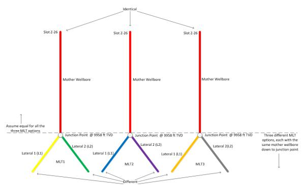
Figure 16: Schematic of the well path configuration. Should only be used for overview. The figure is not to be scaled, and the shown inclinations are incorrect (Figure made by this author)
