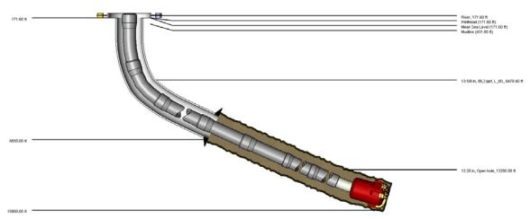
Figure 34: Well schematic for the drilling of the 12 ¼" hole section in the mother wellbore (Wellplan 2013a)
