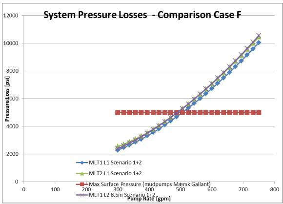
Figure 186: Pressure losses scenario 1 and 2 values comparison case F (Wellplan 2013a)
