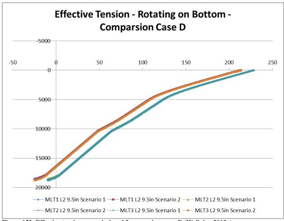
Figure 153: Effective tension scenario 1 and 2 comparison case D (Wellplan 2013a)
