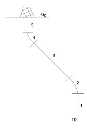
Figure 26: Convenient dividing of the drillstring for manual calculations using the discrete model (Figure made by this author)
