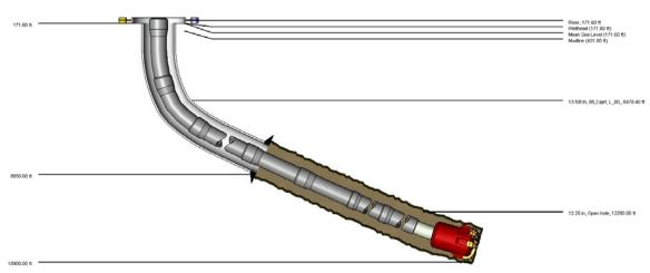
Figure 123: Schematic of hole sections with drillstring for the 12  $^{1}\!\!4$ " drilling in mainbore (to scale) (Wellplan 2013a)
