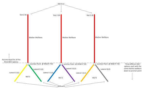
Figure 36: Schematic of the well path configuration. Same as Figure 16. Should only be used for overview. The figure is not to be scaled, and the shown inclinations are incorrect (Figure made by this author)
