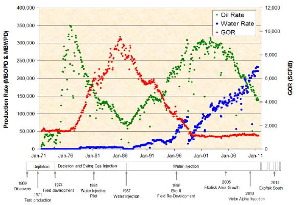
Figure 6: Ekofisk historical production rates, with timeline of significant events since the start in 1971 (ConocoPhillips 2013f)
