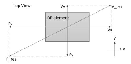
Figure 29: Forces on a drill pipe element with pipe rotation (Figure made by this author)
