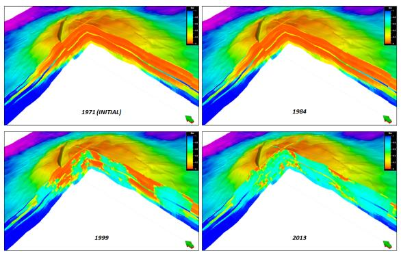
Figure 4: Reservoir model of water saturation in Ekofisk as a function of time (ConocoPhillips 2013h)
