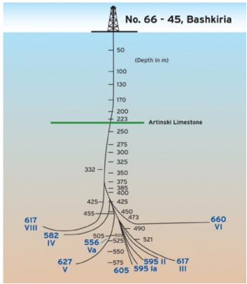
Figure 67: The world's first multilateral well drilled in Soviet in 1953 (E&P Magazine 2007)
