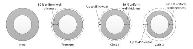
Figure 28: Classification of drill pipes based on wear (Figure made by this author)
