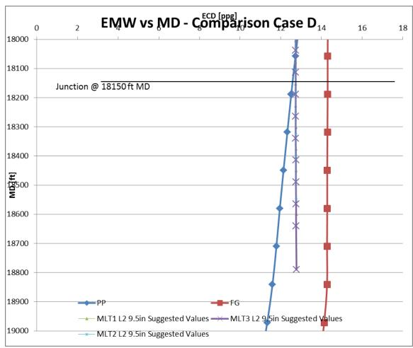
Figure 197: ECD for suggested values comparison case D (Wellplan 2013a)
