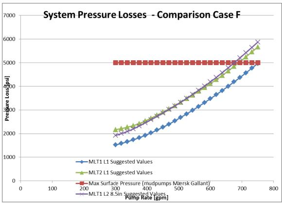
Figure 190: Pressure losses suggested values comparison case F (Wellplan 2013a)
