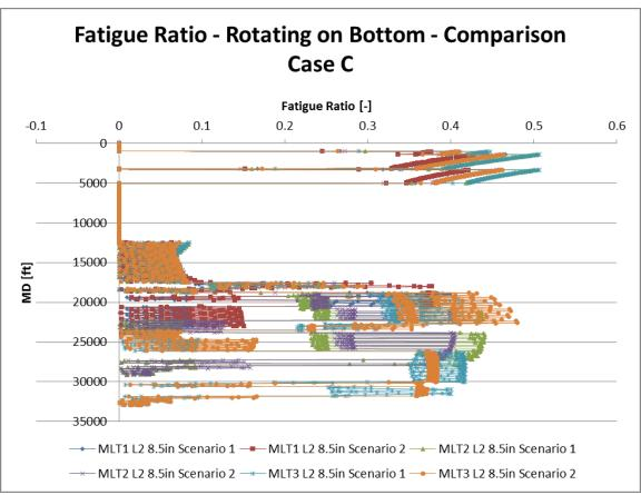
Figure 169: Fatigue ratio scenario 1 and 2 values comparison case C (Wellplan 2013a)
