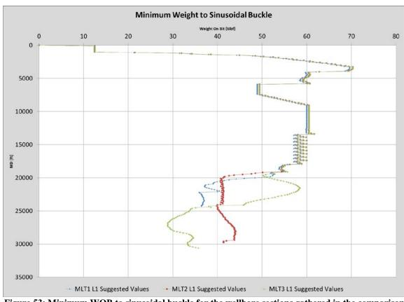
Figure 53: Minimum WOB to sinusoidal buckle for the wellbore sections gathered in the comparison case A for scenario 1 and scenario 2 input parameter values (Wellplan 2013a)
