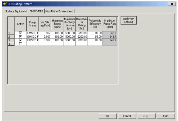
Figure 145: Circulating system setup for both Scenario 1 and Scenario 2 based on Mærsk Gallant specifications (Wellplan 2013)
