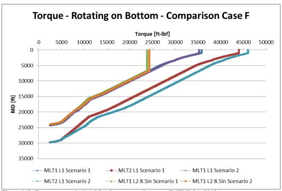
Figure 163: Torque scenario 1 and 2 values comparison case F (Wellplan 2013a)
