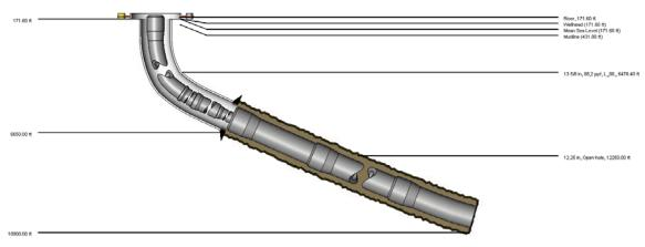
Figure 128: Schematic of hole sections with string for running of 10  $^{3}4$ " liner in mainbore (to scale) (Wellplan 2013a)
