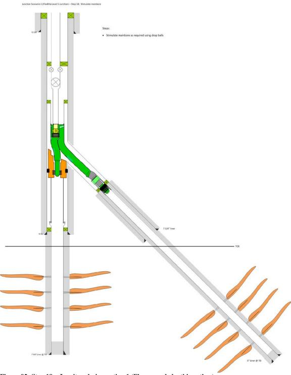
Figure 92: Step 18 – Junciton design option 1 (Figure made by this author)
