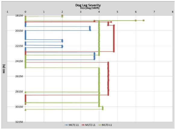
Figure 38: DLS for the wellbore sections compared in comparison case A (Wellplan 2013a)
