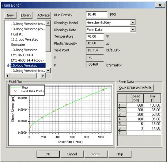
Figure 111: Mud program for the drilling of the 20" x 17 ½" hole section in mainbore (Wellplan 2013a)
