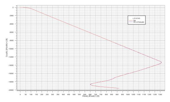
Figure 136: Well path plan view for the drilling of  $9\frac{1}{2}$ " section from junction to TD for MLT1 Lateral 1 (Wellplan 2013)
