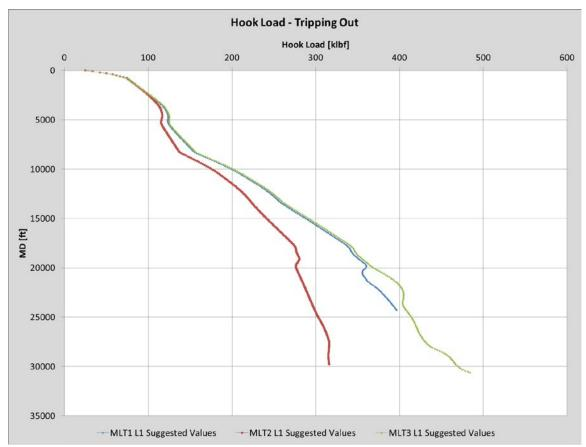
Figure 49: Hook load at surface for bit at different measured depths for the wellbores in comparison case A with suggested input values (Wellplan 2013a)
