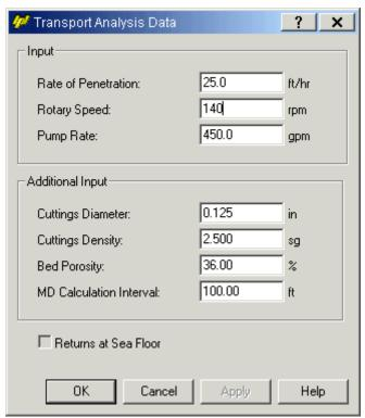
Figure 148: Transport analysis data initial setup for Scenario 1 (Wellplan 2013)
