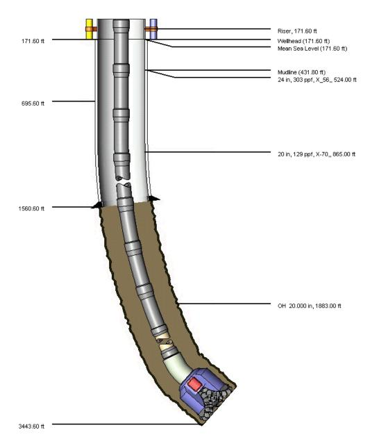
Figure 107: Schematic of hole sections with drillstring for the 20" x 17  $\frac{1}{2}$ " drilling in mainbore (to scale) (Wellplan 2013a)
