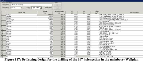
Figure 117: Drillstring design for the drilling of the 16" hole section in the mainbore (Wellplan 2013a)
