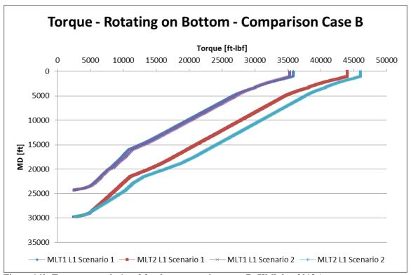
Figure 160: Torque scenario 1 and 2 values comparison case B (Wellplan 2013a)
