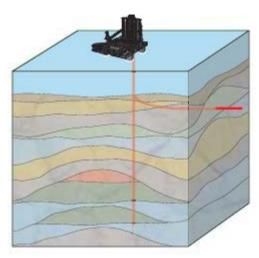
Figure 72: Satellite field being drained by a multilateral well (Frailja et al. 2002)
