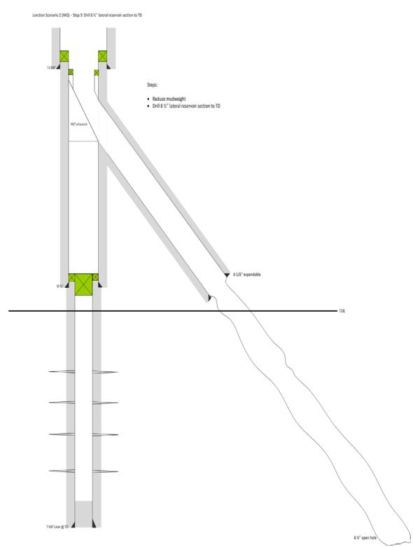
Figure 96: Step 9 – Junction design option 2 (Figure made by this author)
