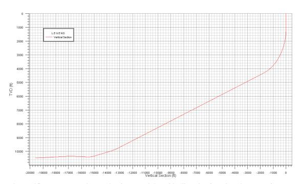
Figure 135: Well path vertical section for the drilling of 9 ½" section from junction to TD for MLT1 Lateral 1 (Wellplan 2013)
