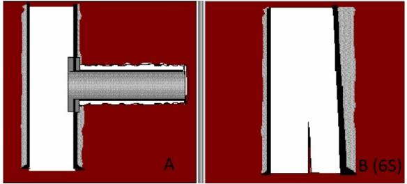
Figure 15: TAML Level 6A and Level 6B (6S) Junctions (Weatherford 2006)
