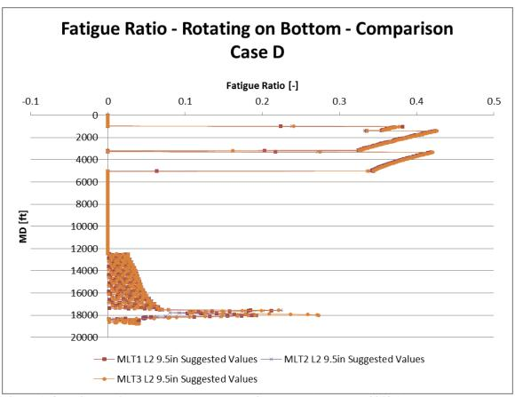
Figure 174: Fatigue ratio suggested values comparison case D (Wellplan 2013a)
