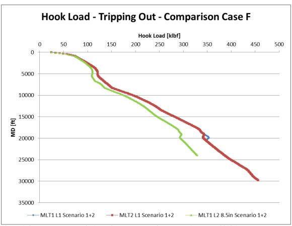
Figure 179: Hook load scenario 1 and 2 values comparison case F (Wellplan 2013a)
