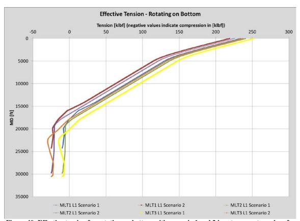
Figure 40: Effective tension for rotating on bottom with scenario 1 and 2 input parameter values for comparison case A (Wellplan 2013a)
