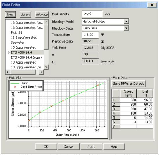
Figure 127: Mud program for the drilling of the 12 1/4" hole section in mainbore (Wellplan 2013a)
