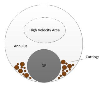
Figure 31: High velocity area in a horizontal well (Figure made by this author)
