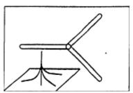
Figure 79: Top and 3D view of a radial tri-lateral, also referred to as a radial fan or chicken foot ML (Crouse 1996)
