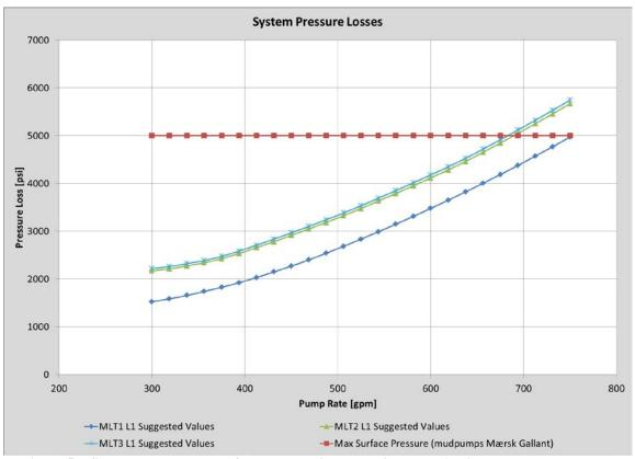
Figure 57: System pressure losses for wellbores in comparison case A with suggested parameter input values (Wellplan 2013a)
