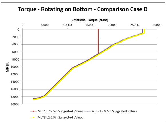
Figure 166: Torque suggested values comparison case D (Wellplan 2013a)
