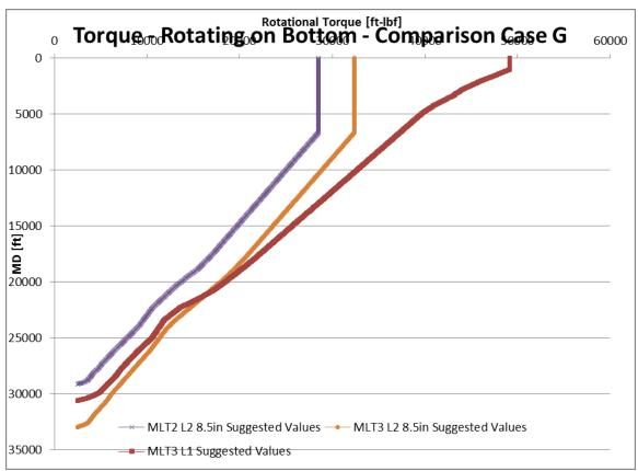
Figure 168: Torque suggested values comparison case G (Wellplan 2013a)
