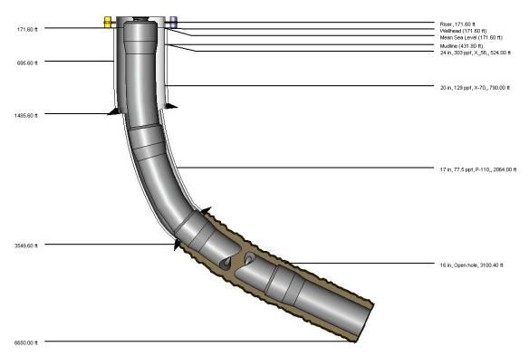
Figure 120: Schematic of hole sections with string for running of 13 5/8" casing in mainbore (to scale) (Wellplan 2013a)
