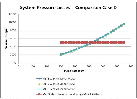
Figure 185: Pressure losses scenario 1 and 2 values comparison case D (Wellplan 2013a)
