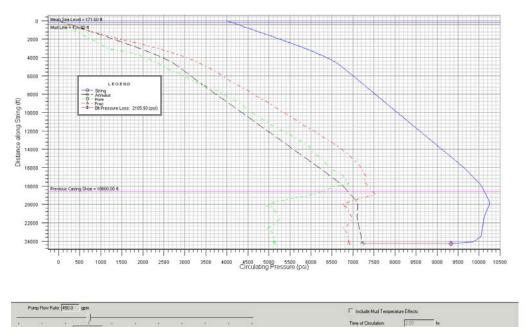
Figure 58: Circulating pressure for MLT1 L1 for scenario 1 parameter input values (Wellplan 2013a)
