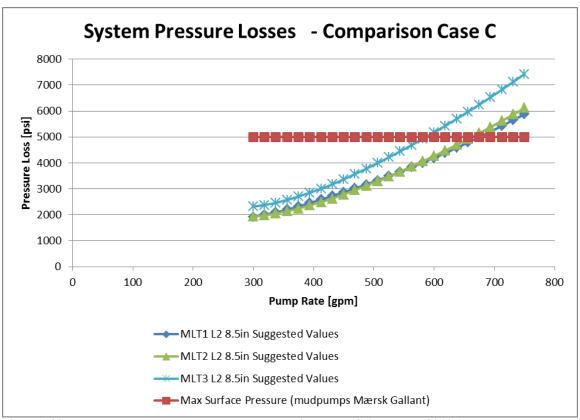
Figure 188: Pressure losses suggested values comparison case C (Wellplan 2013a)
