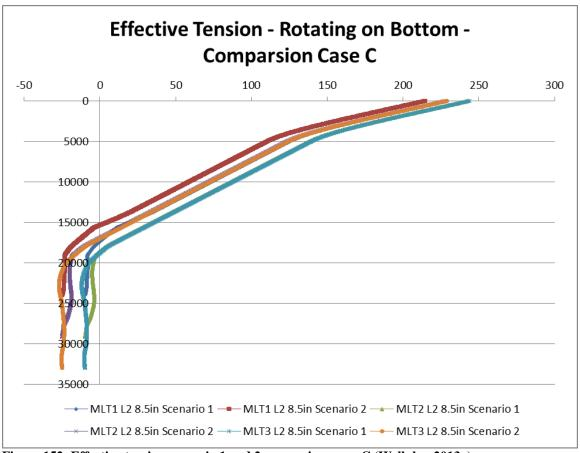
Figure 152: Effective tension scenario 1 and 2 comparison case C (Wellplan 2013a)
