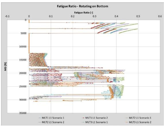
Figure 46: Fatigue ratio for comparison case A with scenario 1 and scenario 2 input parameter values (Wellplan 2013a)
