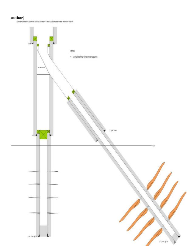
Figure 88: Step 12 – Junciton design option 1 (Figure made by this author)
