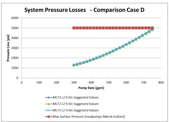
Figure 189: Pressure losses suggested values comparison case D (Wellplan 2013a)
