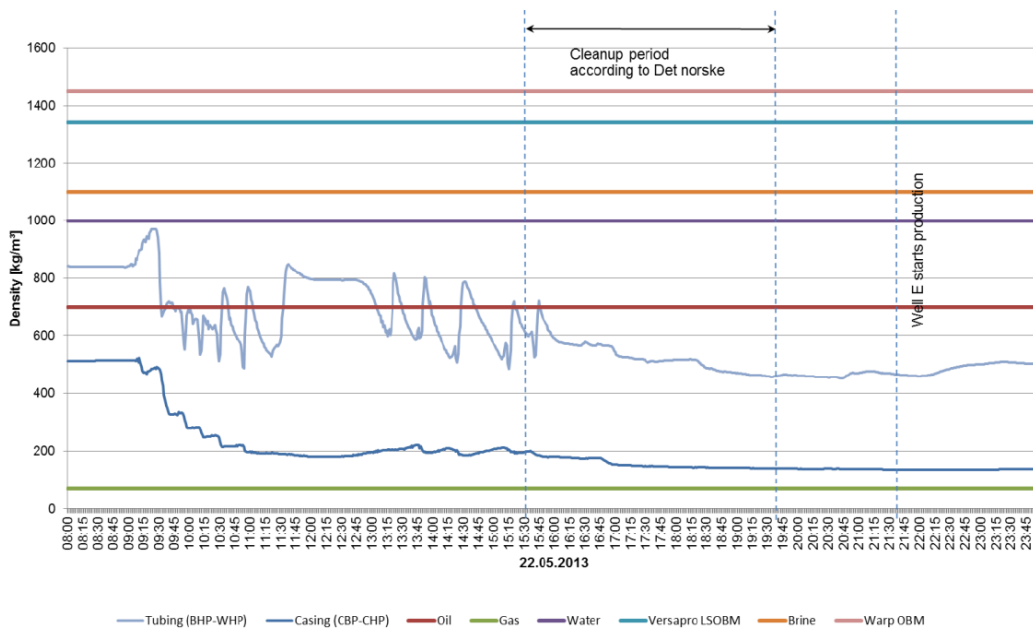
Figure 6.9: Density of fluid in tubing (BHP-WHP) and annulus (CBP-CHP) between wellhead and P/T-gauge compared to densities of fluids in Well D at start of clean-up, from Lysne & Nakken (2013), page 25.
