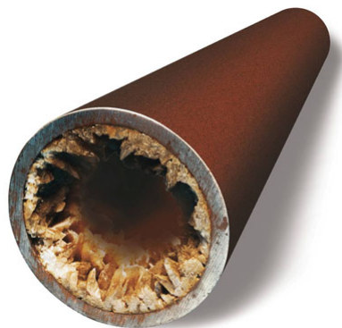
Figure 5.10: Scale can severely impede flow by clogging perforations or forming a thick lining in the production tubing, from Schlumberger (2014 l ).
