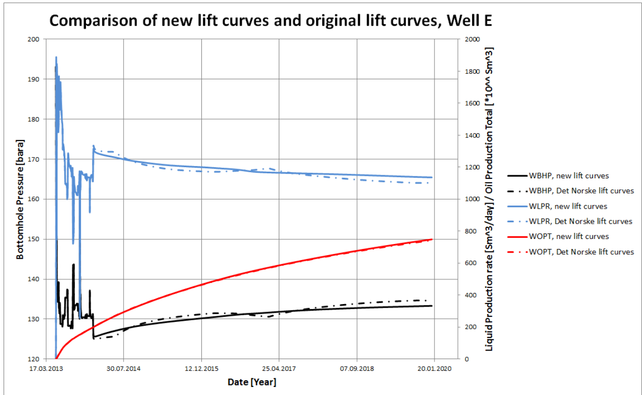
Figure 9.4: Comparison of the new lift curves and the original lift curves by Det Norske Oljeselskap. Well E. The black lines show the BHP, the blue lines show the liquid production rate and the red lines show the total oil production.
