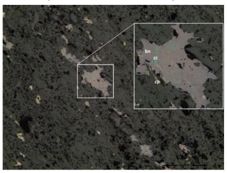
Figure 46. Photomicrograph of thin section NUS\_031 in drill core NUS-DD-13-003, in reflected light. It shows an example of mineralization in the Lower mineralized horizon. Bornite (bn), chalcopyrite (cp) and chalcocite (cc) occured as disseminated grains and in veins. Chalcopyrite (cp) and chalcocite (cc) formed inclusions in the bornite grain (bn). Photo: Kjersti Moen.
