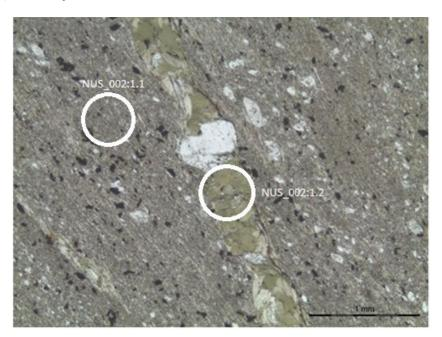
Figure 48. Picture of the hang wall slate in thin section NUS\_002, in plan polarized light. White circles mark the selected spot in the matrix (NUS\_002:1.1, No. 5-12) and mineral grains (NUS\_002:1.2, No.2-4). Photo: Kjersti Moen.
