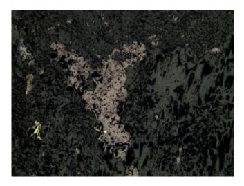
Figure C105. Mineralization of bornite and chalcopyrite in the Upper mineralized horizon. Picture taken by reflection light in thin section NUS\_005 in drill core NUS-DD-13-004. The picture represents the opaque part in the left part of Figure C104.
