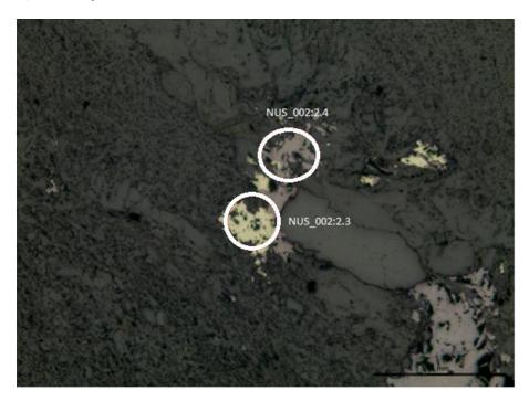
Figure 58. Picture of hang wall slate in thin section NUS\_002, reflected light. White circles mark the analysed spot of minerals (selected spot, NUS\_002:2.3, No. 19-21, and NUS\_002:2.4, No. 22-24). Photo: Kjersti Moen.
