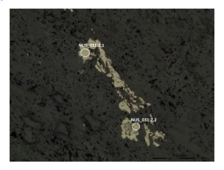
Figure 74. Photomicrograph show analyse area NUS\_031:2 (Figure 72) in thin section NUS\_031 in the Upper mineralized horizon in drill core NUS-DD-13-012. White circles mark the analysed sulphide grains (NUS\_031:2.1, No. 164-166, and NUS\_031:2.2, No. 167-169). Photo: Kjersti Moen.
