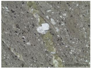
Figure C103. Picture of hang wall slate in thin section NUS\_002. Mica-rich matrix form a schistose texture.
