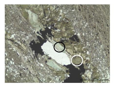
Figure 49. Picture of hang wall slate in thin section NUS\_002, plan polarized light. Circles mark the analysed spot of minerals (selected spot, NUS\_002:2.1, No. 13-15, and NUS\_002:2.2, No. 16-18). Photo: Kjersti Moen.
