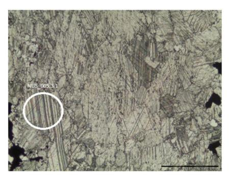
Figure 54. Picture of the Upper mineralized horizon in thin section NUS\_005, plan polarized light. White circle mark the analysed spot of minerals (selected spot, NUS\_005:3.1, No.52-54). Photo: Kjersti Moen.
