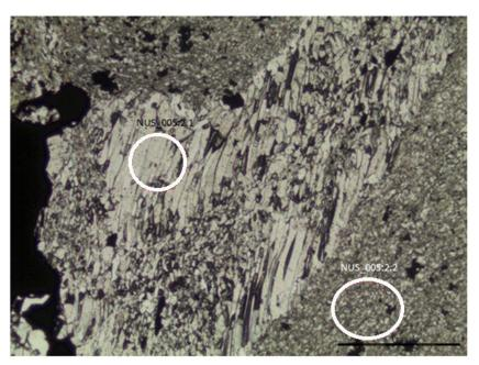
Figure 53. Picture of the Upper mineralized horizon in thin section NUS\_005, plan polarized light. White circles mark the analysed spot of minerals (selected spot, NUS\_005:2.1, No.40-42, and NUS\_005:2.2, No.43-49 and 51). Photo: Kjersti Moen.
