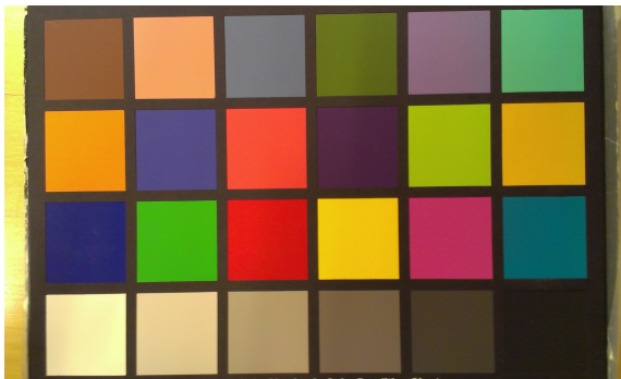
Figure 2.5: Image of the Macbeth ColorChecker used in this project. This image was taken using an HTC One V with the fluorescent white balance setting. The light source was a combination of fluorescent light bulbs and daylight.
