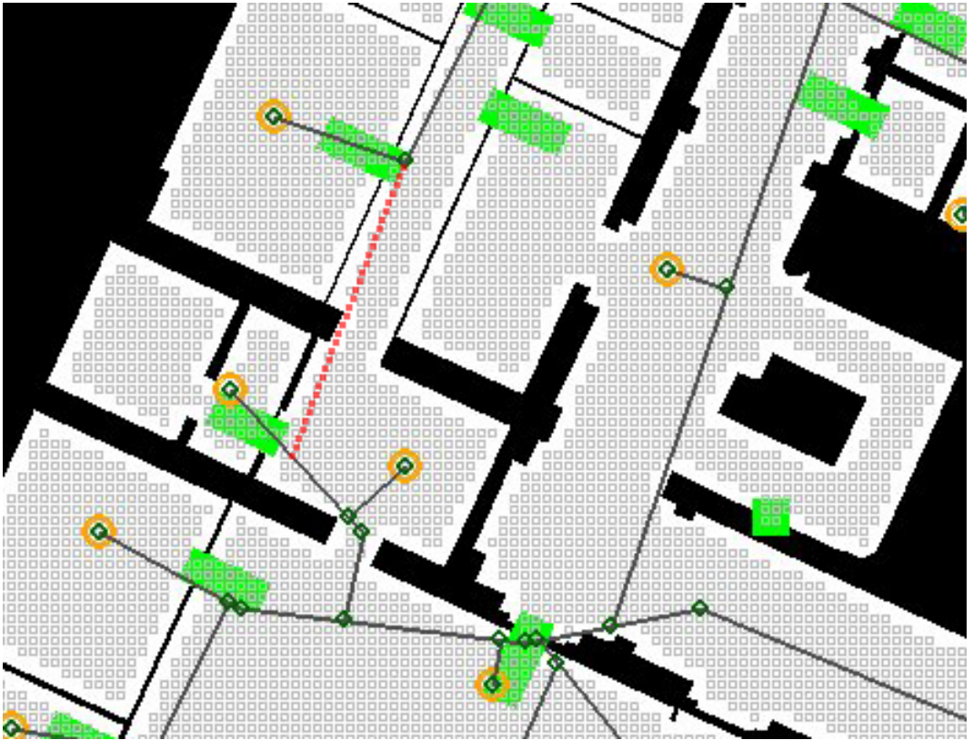
Figure 6.4: Lack of connections: while manually creating paths, we would have added a line where we have drawn the red dotted line now.
