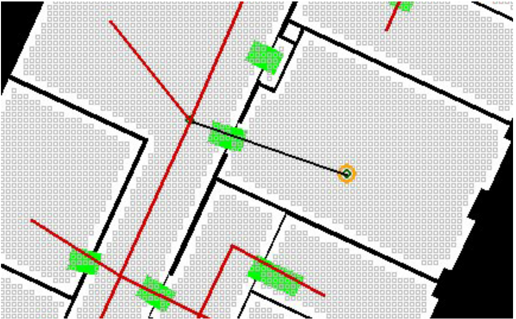
Figure 6.1: Connecting a new path to already existing paths. Lines coloured red are already existing paths, the black line is a new generated path.
