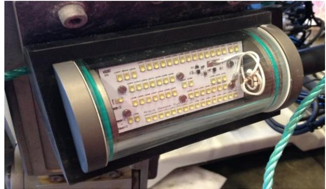
FIGURE 48: DEEPWATER LAMPS ON AN ARGUS ROV
