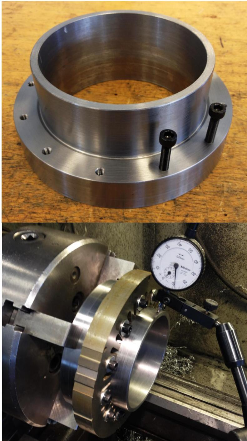
FIGURE 81: STATOR JIG BEFORE AND AFTER MOUNTING IN THE LATHE
