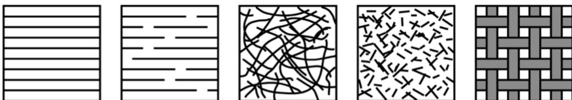
FIGURE 104: FIBRE ORIENTATION IN COMPOSITES - FROM LEFT: UNIDIRECTIONAL CONTINUOUS AND DISCONTINUOUS, RANDOMLY ORIENTED LONG AND SHORT FIBRE AND WEAVED FABRIC [44]
