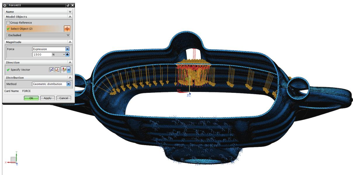
FIGURE 134: HULL LOAD STATE
