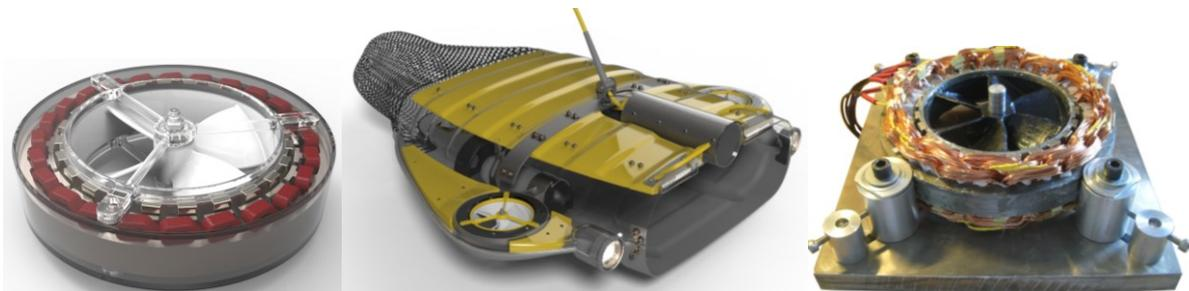
FIGURE 1: LATEST RIM-THRUSTER DESIGN (LEFT) AND FINAL ROV RENDERED WITH A TRANSLUCENT CASING (MIDDLE) AND RIG MOUNTED THRUSTER PROTOTYPE (RIGHT).
