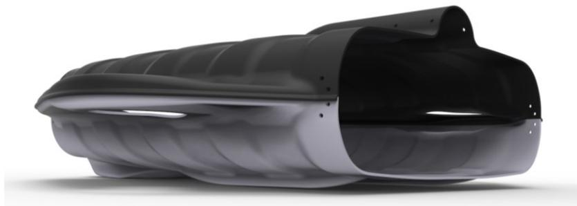
FIGURE 14: CORRUGATED HULL
