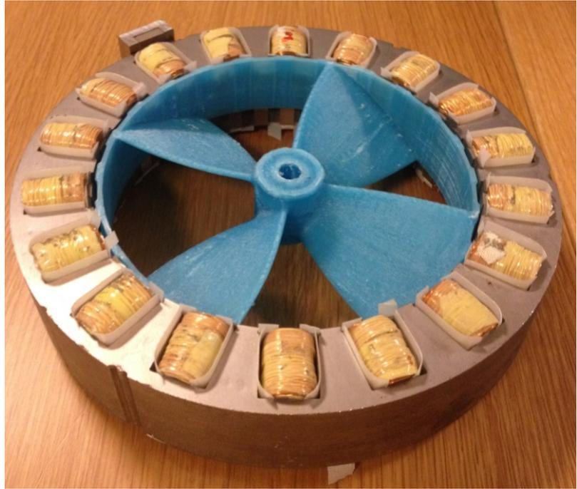
FIGURE 79: SMART MOTOR ACTUATOR STATOR
