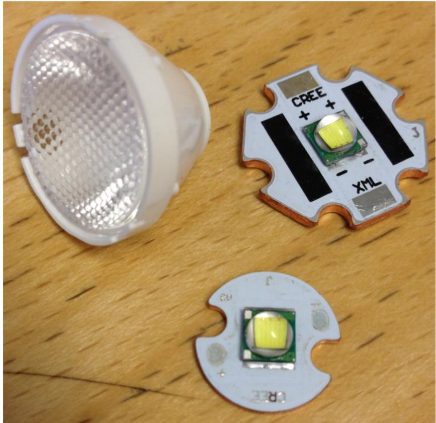
FIGURE 55: 60° LENS (UPPER LEFT), 20MM XML LED (TOP) AND 16MM (BOTTOM)
