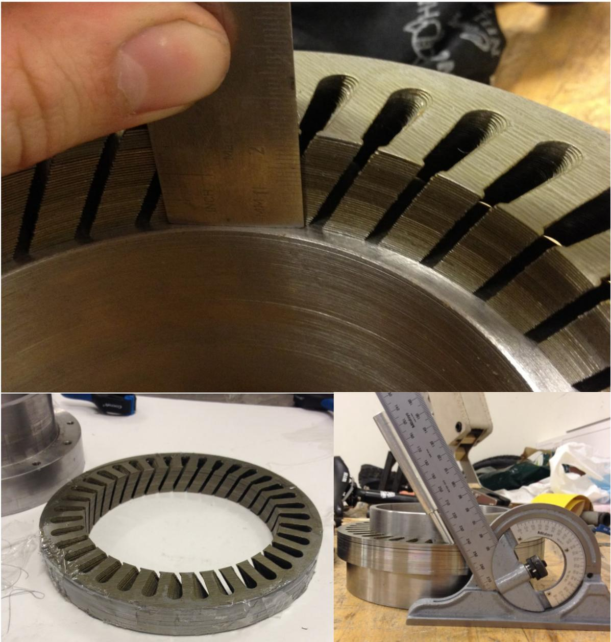
FIGURE 83: SKEWING OF THE STATOR TEETH
