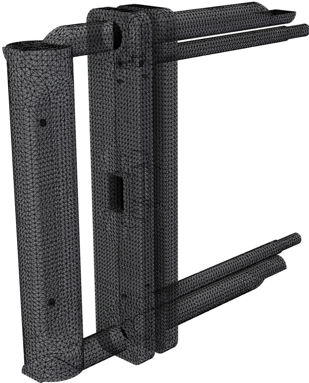
Figure 11-7 EDS meshed model
