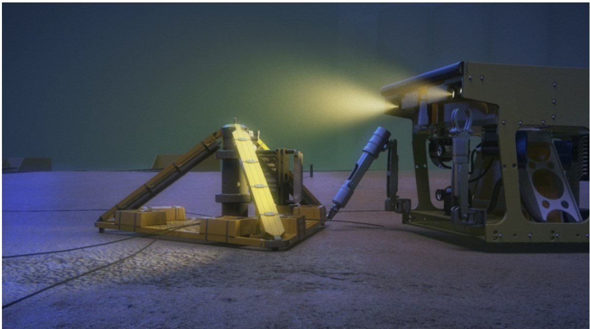
Figure 9-7 SCS, view during ROV deployment
