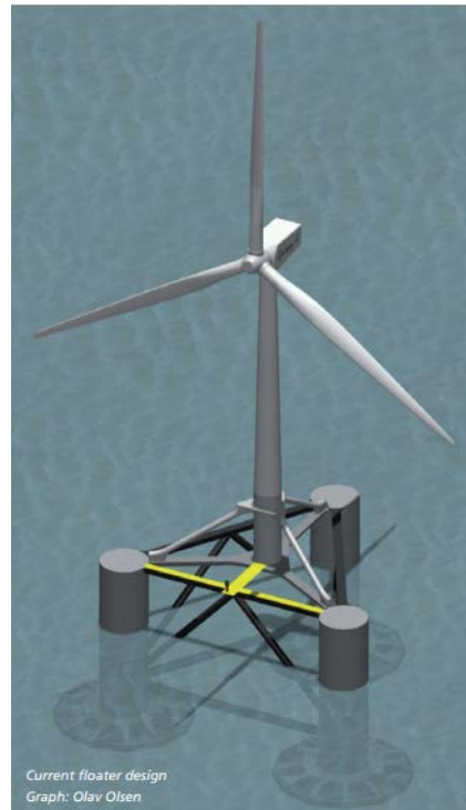
Figure 5 HiPrWind floating windturbine structure, picture from (HiPRWind, 2011)
