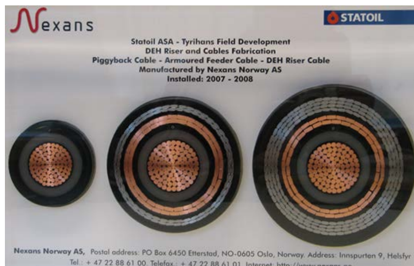
Figure 6: Cross-section of cables used for the DEH installation at the Tyrihans field [18]
