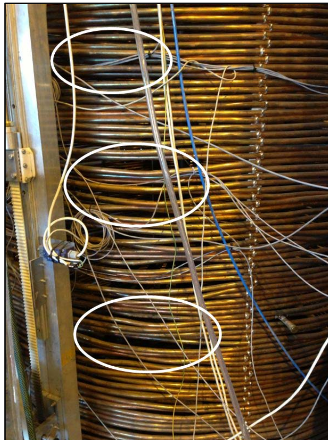
Figure 48: Copper tubing with uneven pitch
