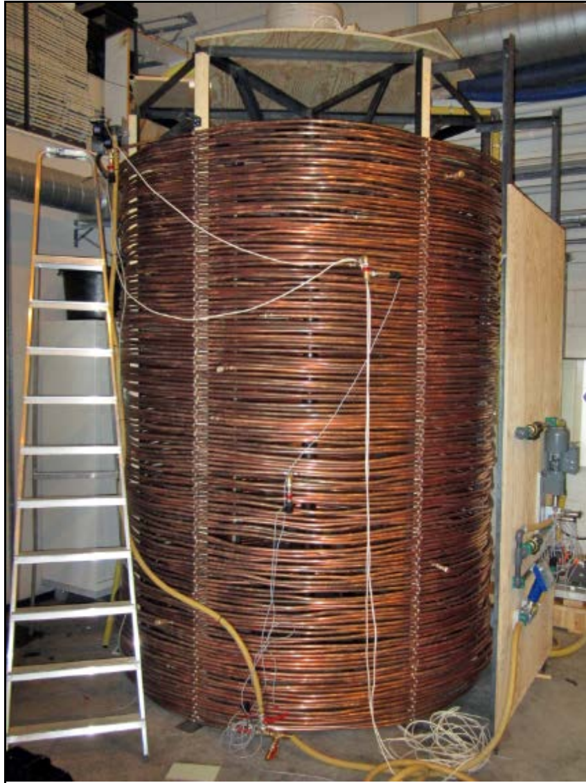
Figure 39: Actual picture of copper tubing coil
