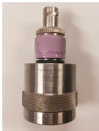
(a) Olympus IMS 1 MHz Immersion Transducer.
