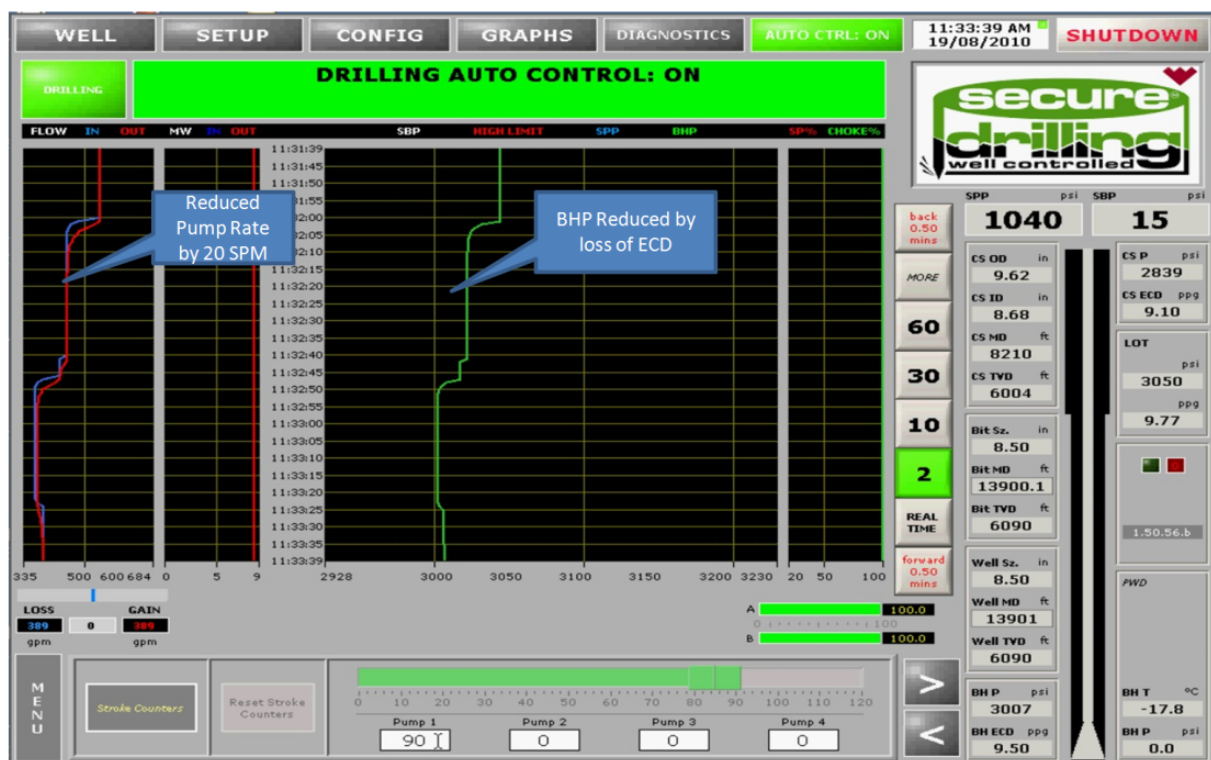
Figure 21: Defining the lower end of the operational envelope. The red line shows flow out, the blue line flow in and the green line shows the current BHP. Additionally the specific amount mud lost or gained are shown in the lower left side of the control screen (Weatherford 2013)
