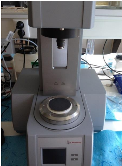
Figure 12 MCR 302 rheometer with static plate cell
