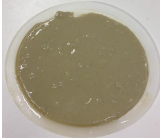
Figure 20 Filter cake of OMB with 5% bentonite, 9% methanol and 1% 16nm ow particles
