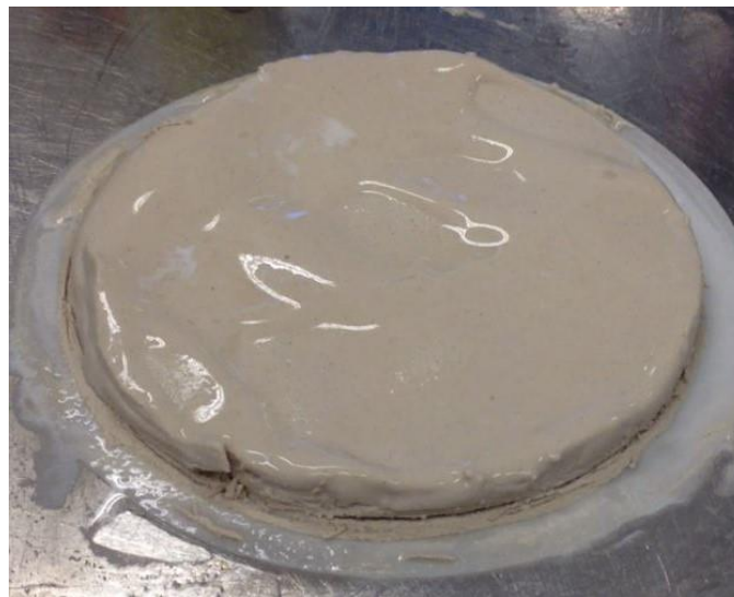
Figure 14 Filter cake of 5 wt% oil wet particle in WBM
