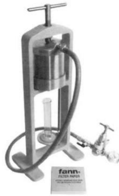
Figure 3.19: Filter Press, Standard Frame, W/ Regulator
