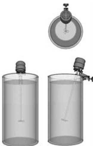
Figure 3.2: Vortexing Installation of the mixer
