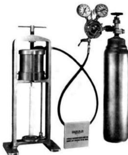
Figure 3.11: Filter Press with Nitrogen Cylinder Pressure Source
