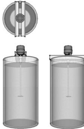
Figure 3.3: High Speed Mixer shaft installation
