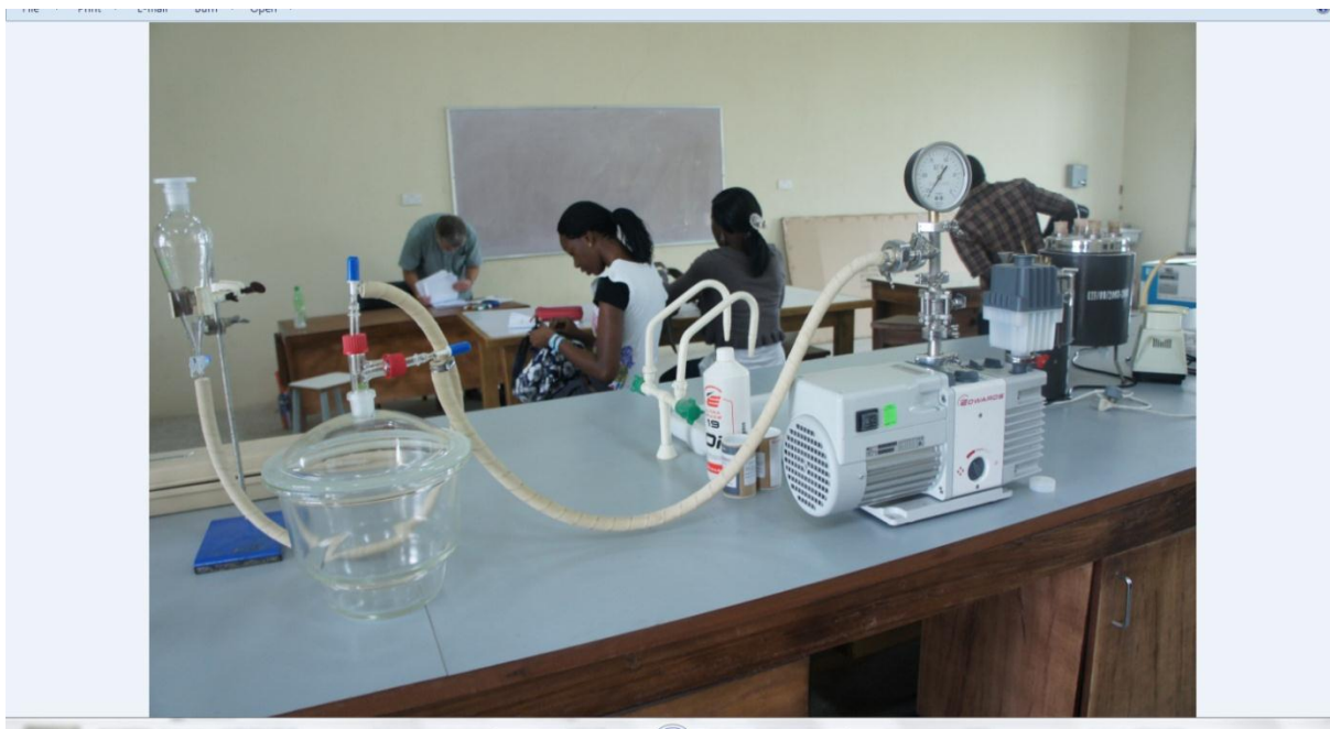
Figure 8: Desiccator and accessories, vacuum pump and accessories, vacuum gauge, Oil Mist Filter EMF 10 plus filter, EMF 10 Spare Mist Element, Ultra Grade 19 Oil, connection tubes and fittings
