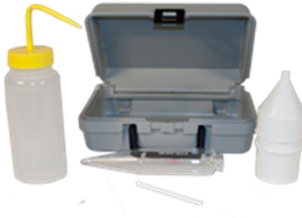
Figure 3.9: The sand content kit and its parts
