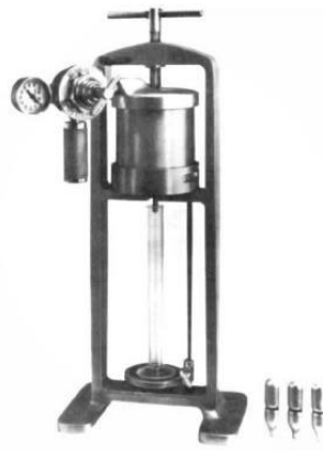
Figure 3.20: Filter Press, Standard Frame, W/ CO2 Pressure Source
