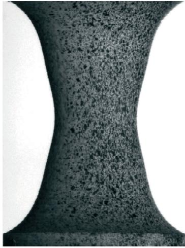
**Figure 5.5: Representative image from tension test performed on a circular HDPE sample.**
