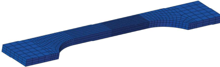
**Figure 7.29: Mesh for simulations of rectangular PVC samples in uniaxial tension.**
