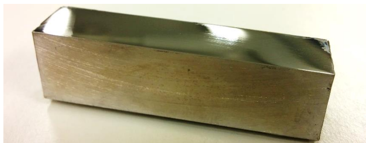
Figure 20: Cross-section polished to mirror quality.
