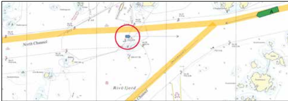
Figure 2: A small eastbound craft (in the red circle) would need to know the intentions of the autonomous unmanned westbound vessel A: will it continued straight, or turn port for the South Channel?
