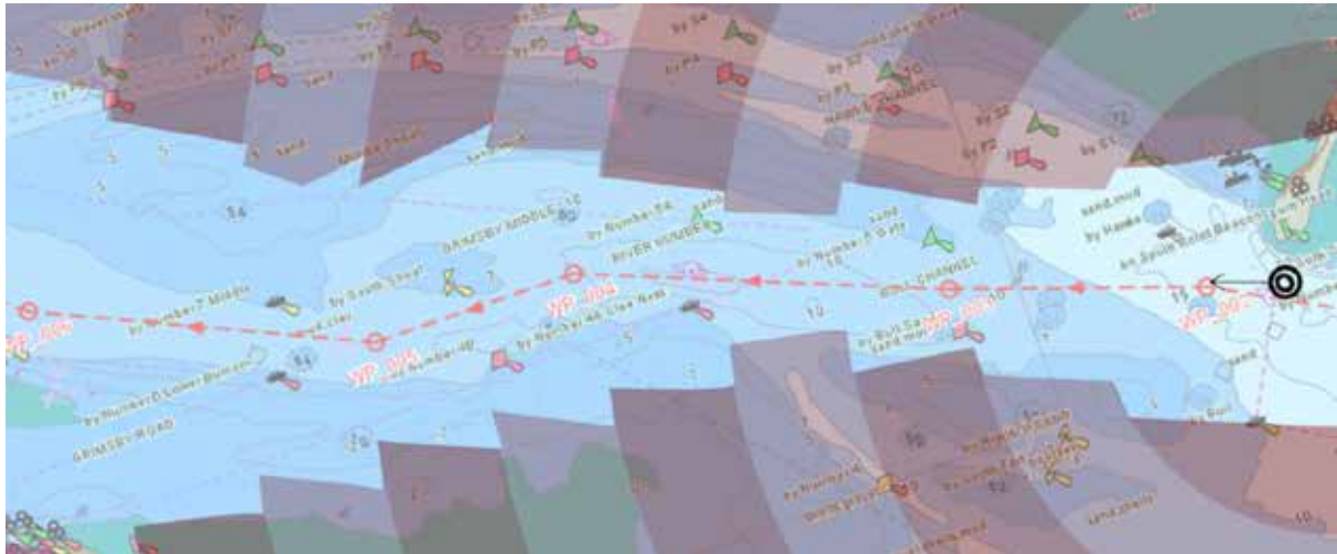
Figure 8. A time dependent NoGo area might look something like this. It is generated automatically in front of the ship and does not only take ships draught into consideration, but also the tidal situation at a particular point along the ships future route at the time the ship will be there. The time segments could for instance be 30 minutes.
