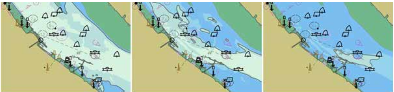
Fig. 2. The water area outside Immingham oil terminal in an electronic chart. The safety contour is set to 2 (left), 5 (middle), and 10 meters (right). The contours needs to be available in the chart database, so, for instance, a safety contour of 8.5 meters cannot be set: it will instead be the next deeper contour, 10 meters.
