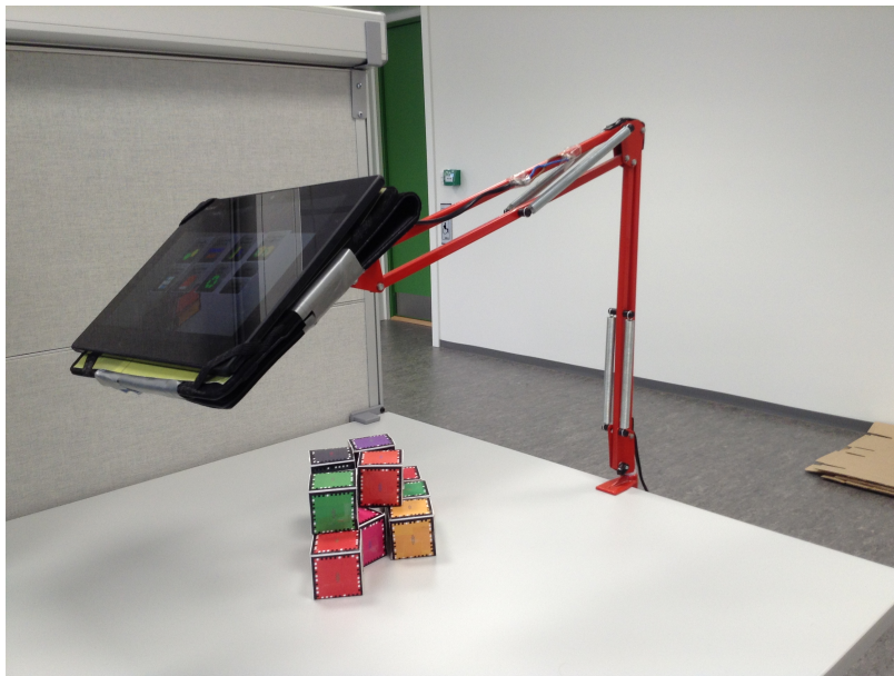
Figure 12.2: The CogARC interaction setup: the 10 cubes and the tablet PC on the base stand.
