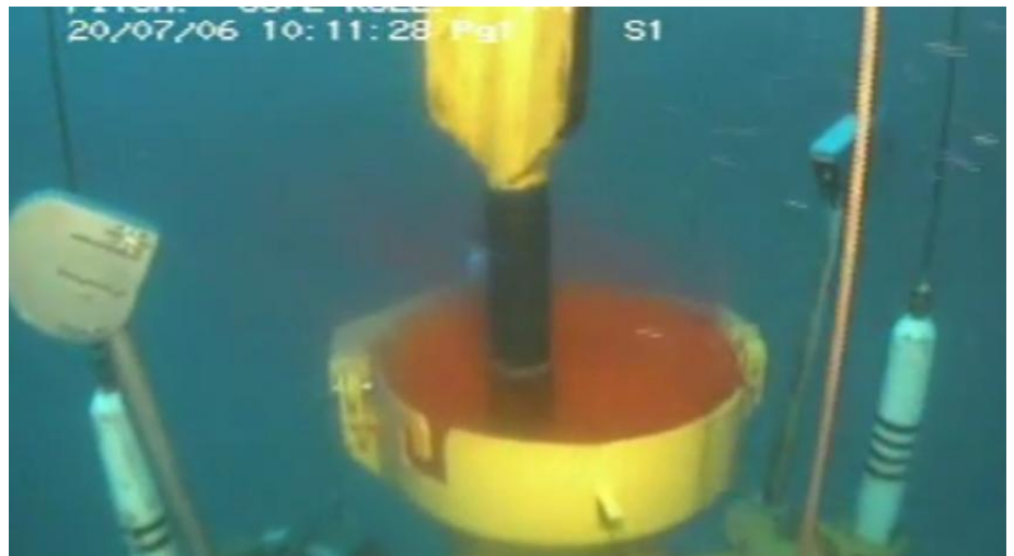
Figure 6: Drillstring being lowered into the SMO
