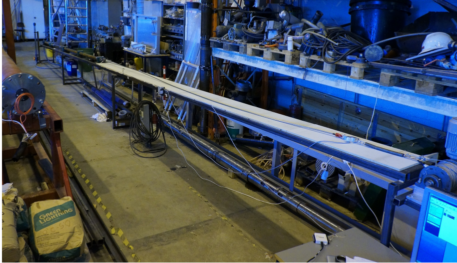
Figure 13: An overview of the laboratory set up. In this picture, the drill string has been pulled out of the annulus.
