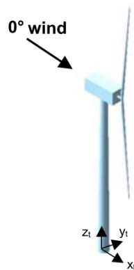
Fig. 2.5: Main coordinate system used in FAST, shown on a downwind turbine (Jonkman and Buhl, 2005)
