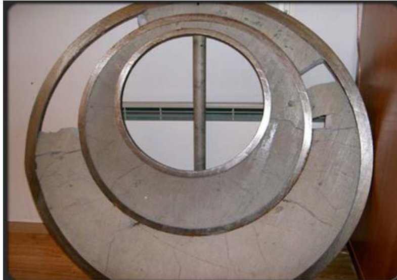
FIGURE 14 : RADICAL CRACK CAUSED BY OIL HEATING (43)
