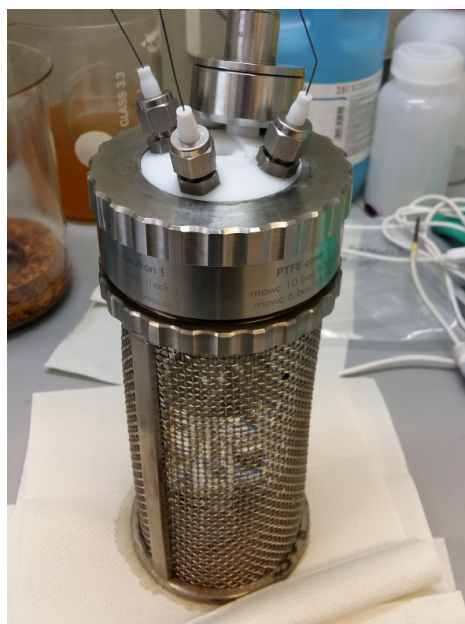
Figure 3.1: The full autoclave setup with three electrodes and manometer.
