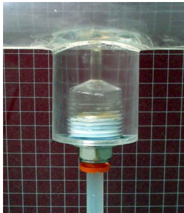
Figure 2.18: Pressure tap at the pipe bottom.
