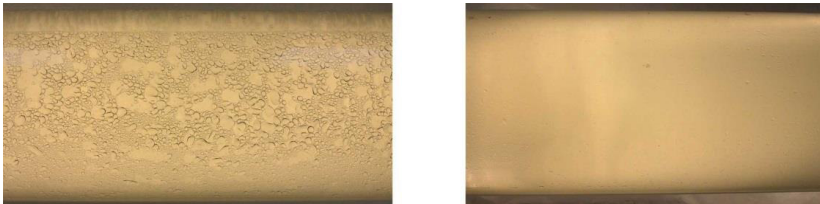
Figure 2.21: Pipe before (left) and after cleaning (right).
