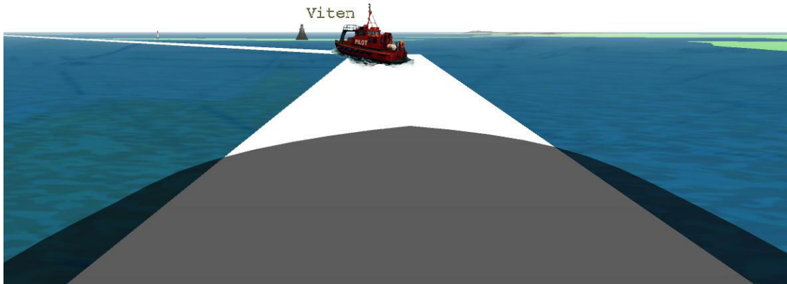
Figure 5. Keep your distance to the virtual pilot boat. This could be a simple and intuitive way of requesting a specific speed for the ship under pilotage.
