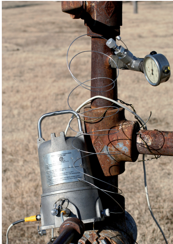
Fig. 1.1 – The SPIDR unit mounted on a well during a well test. The center cable is used for communication with a laptop computer, the left cable connects to the DP cell, and the spiral tube to the right is used to measure tubinghead pressure.
