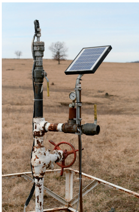
Fig. 2.33 – The wellhead of the Boyd Cable #2. Wires from the temperature probes exit the well through the swab valve. A solar panel is mounted on the well, to power the temperature logger.
