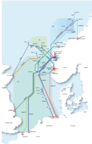
Figure 1: Overview of the Norwegian natural gas transport system in the North Sea which Gassco operates. Figure courtesy of Gassco.
