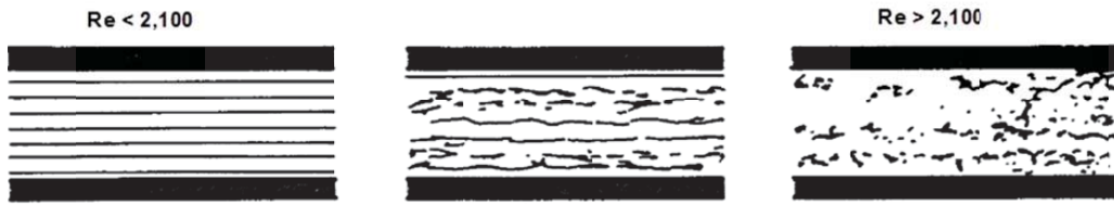
Figure 5.14a,b,c:(a) Laminar flow. (b) Transition between laminar and turbulent flow. (c) Turbulent flow.
