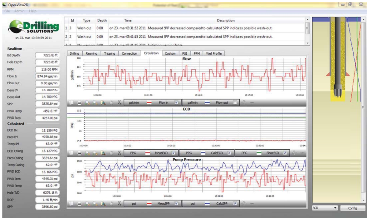
Figure 5.1: The 2D-client monitors the drilling process continuously in real-time.
