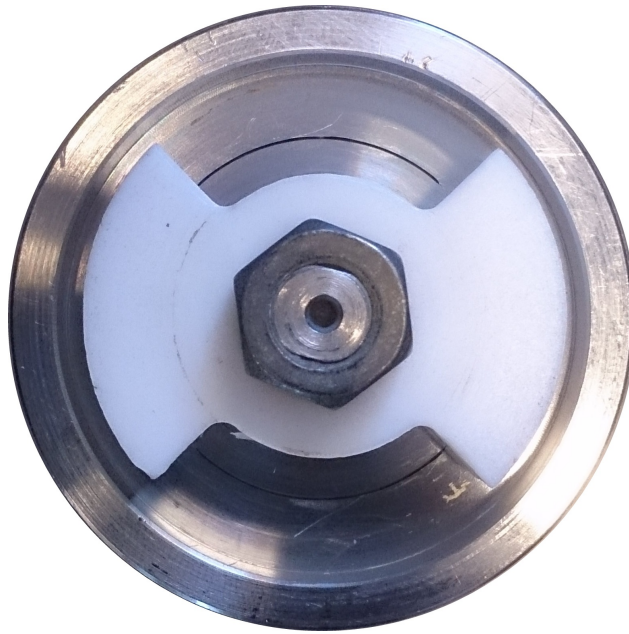
Figure 1.2: The HeaveLock valve in the open position. The cross sectional flow area can be changed by rotating the covering disc.
