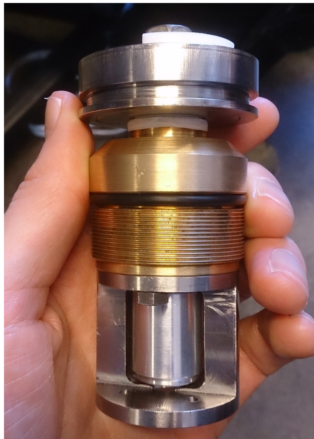
Figure 1.3: The HeaveLock valve as seen from the side. The bottom section is where the motor and gear will be connected to the valve.
