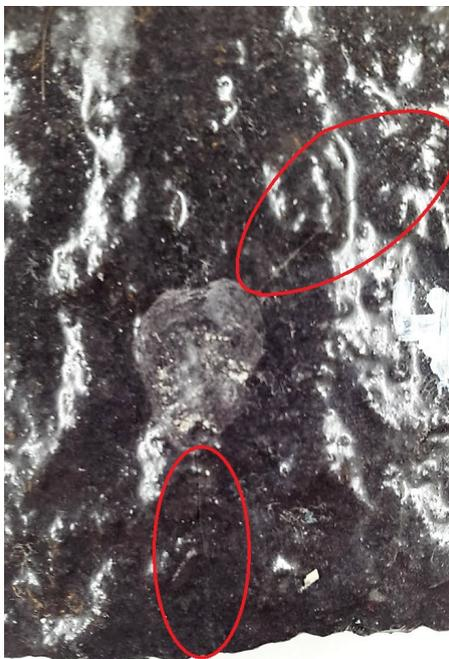
FIGURE 6.34: Coating 4 at -65°C, cracks
