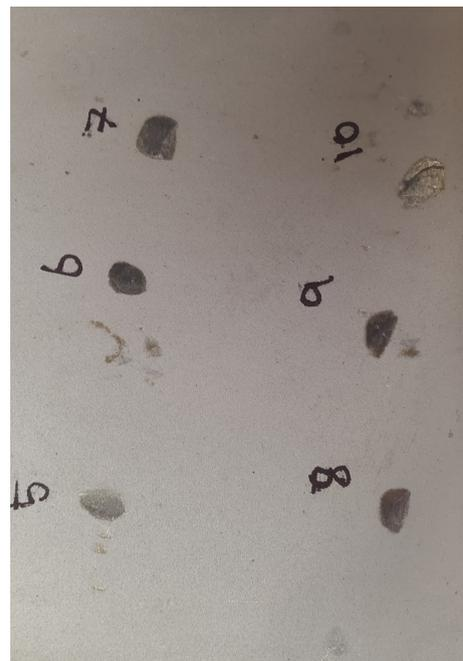
FIGURE 6.15: Coating 1 at -65°C, inclined
