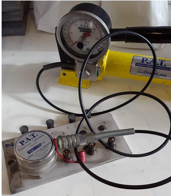
FIGURE 5.2: Pull-off test apparatus
