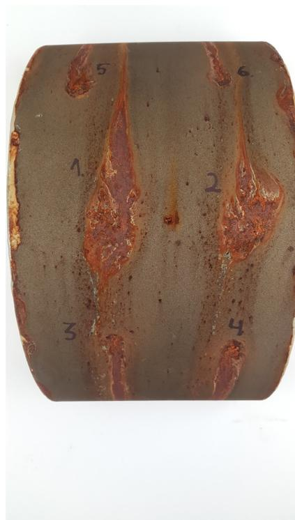
FIGURE 6.39: Coating 2 after corrosion test
