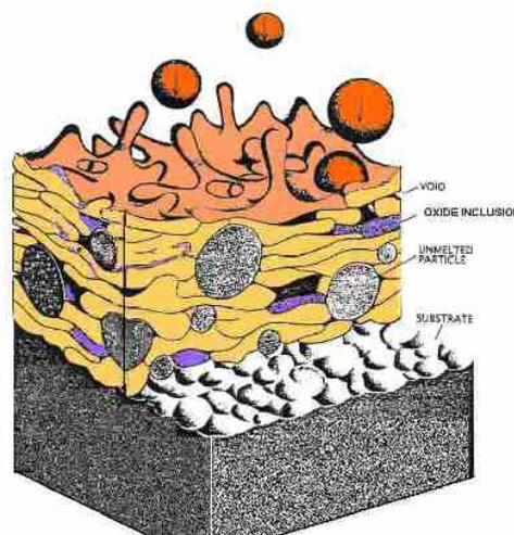
FIGURE 3.2: General Thermal Spray Coating build-up on the substrate
