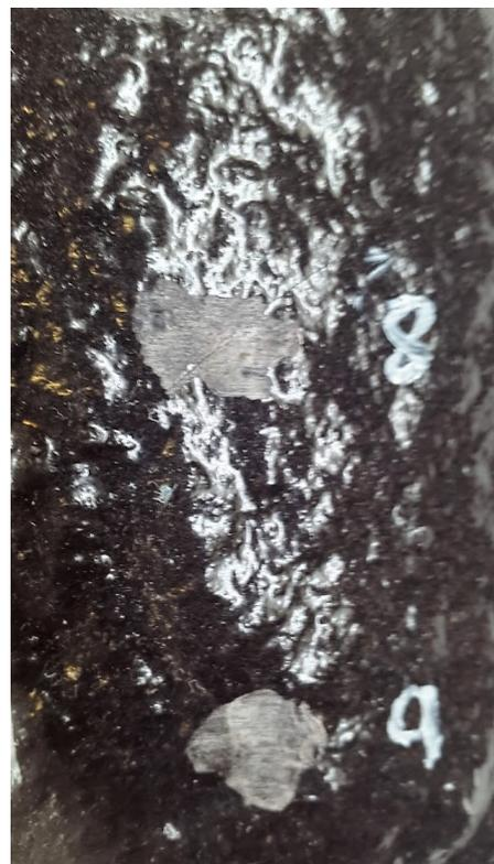
FIGURE 6.35: Coating 4 at -65°C, Cracks
