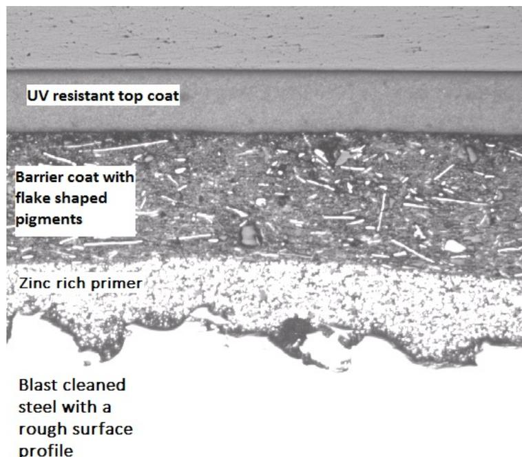
FIGURE 3.1: Example of a 3-layer organic coating system [2]
