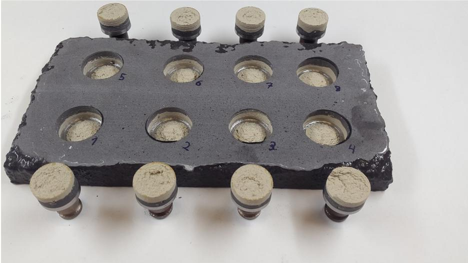
FIGURE 6.7: Coating 4 after adhesion test
