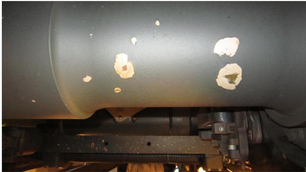
FIGURE 1.1: Impact damages on an axle
