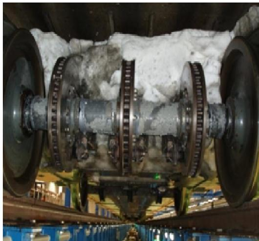
FIGURE 2.2: Ice formation under the train vehicle [1]
