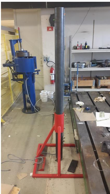
FIGURE 5.4: Impact test apparatus
