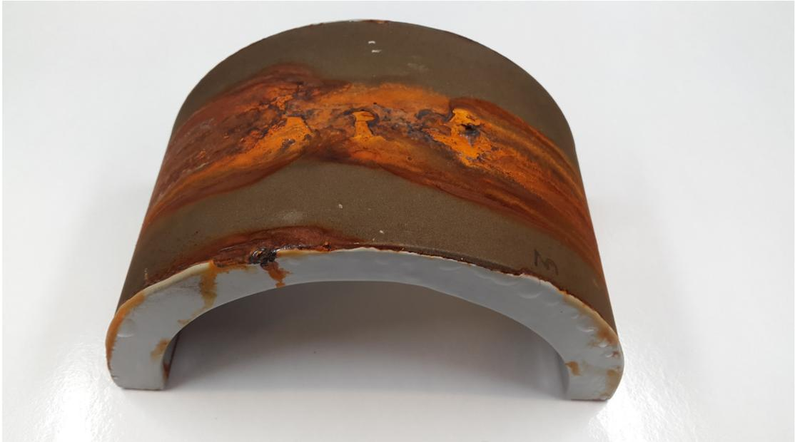
FIGURE 6.45: Coating 2 after 720 hours in the salt spray test
