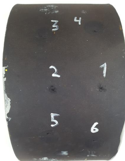
FIGURE 6.41: Coating 3 after corrosion test
