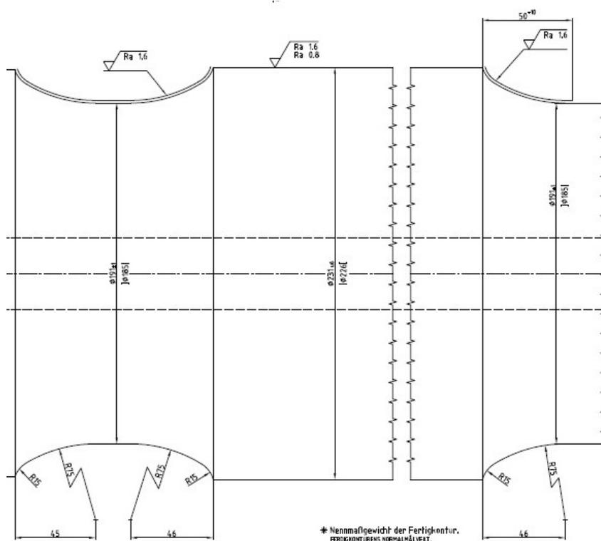
FIGURE 2.1: Technical drawing of an axle with requirements to surface finish
