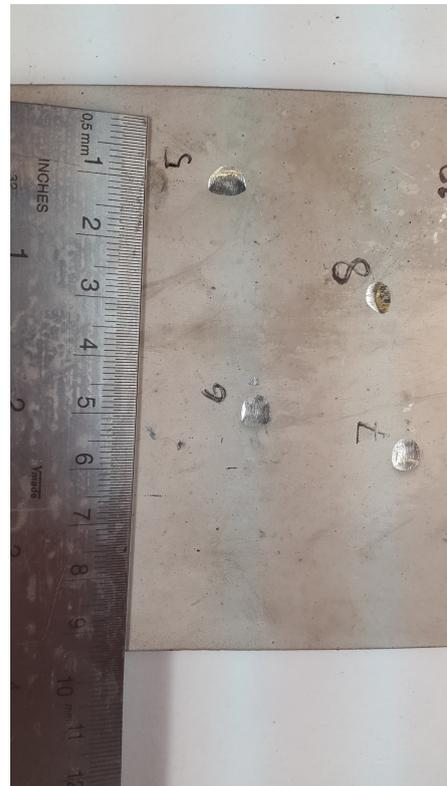
FIGURE 6.13: Coating 1 at -25°C, details
