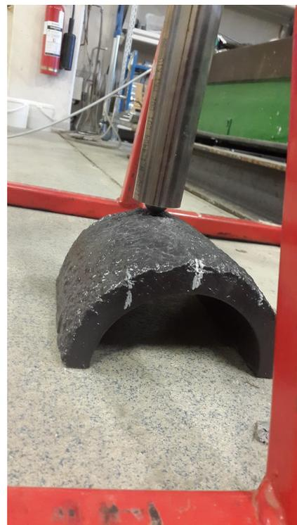
FIGURE 5.5: Impact test apparatus detail
