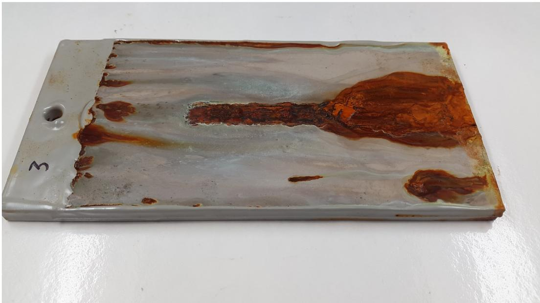
FIGURE 6.44: Coating 1 after 720 hours in the salt spray test
