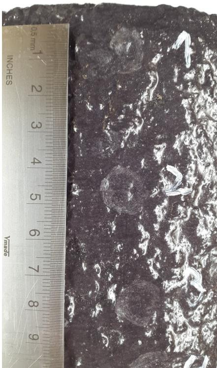
FIGURE 6.32: Coating 4 at -25°C, flat impact
