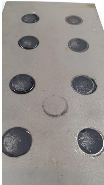
FIGURE 6.4: Fracture surface of Coating 2
