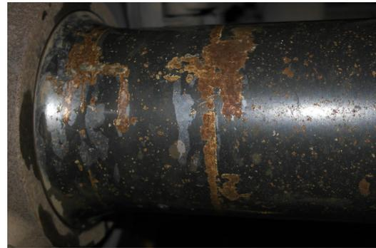
FIGURE 1.2: Corrosion on an axle
