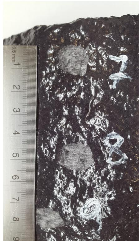
FIGURE 6.33: Coating 4 at -25°C, incline impact
