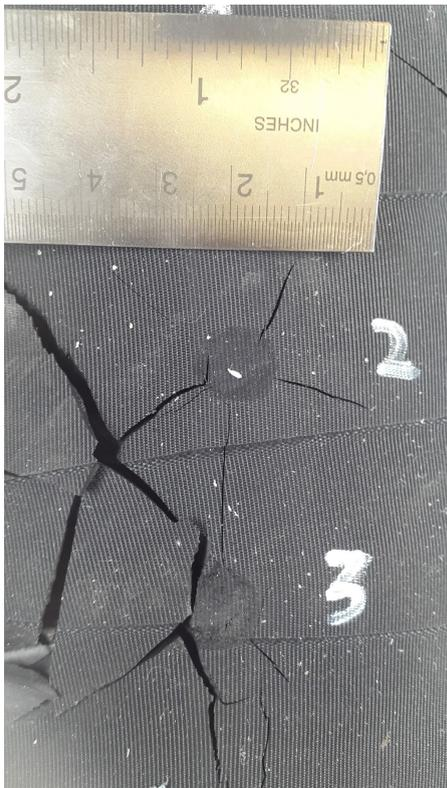
FIGURE 6.28: Coating 3 at -65°C, impact 2,3
