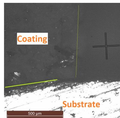
FIGURE 6.51: Coating 4, no corrosion underneath the coating
