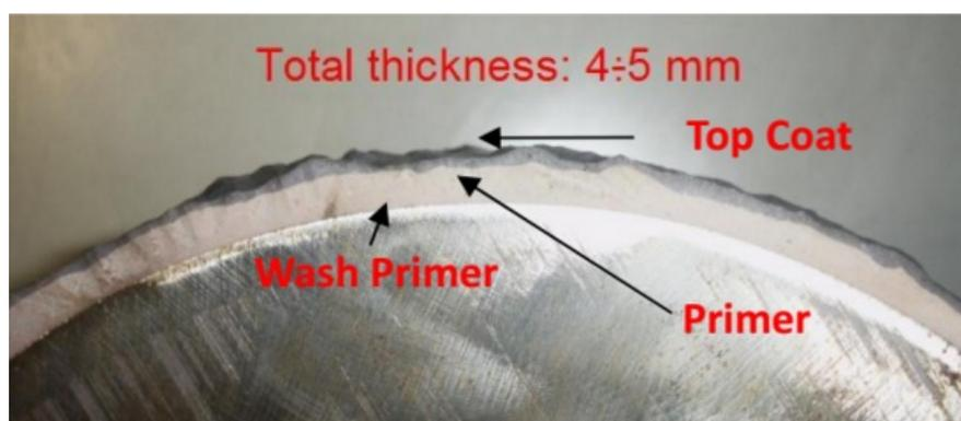
FIGURE 4.1: Cross section view of Lurask
