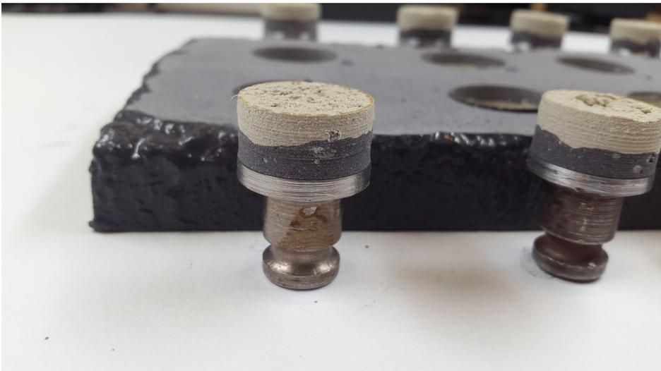
FIGURE 6.8: After adhesion test detail
