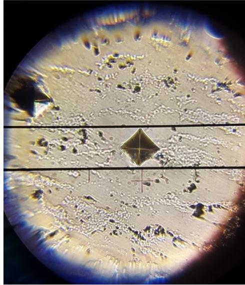
FIGURE 6.1: Hardness measurement of Coating 2 in the cross section
