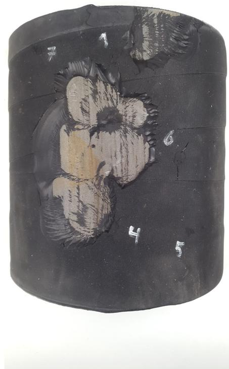
FIGURE 6.29: Coating 3 at -65°, damage
