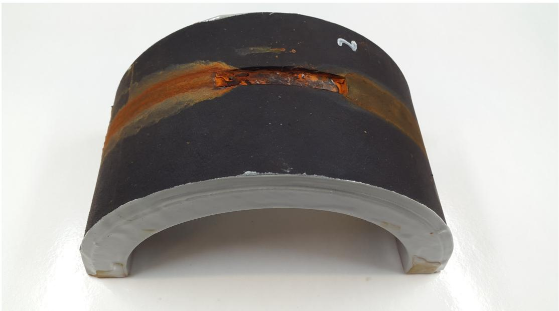
FIGURE 6.46: Coating 3 after 720 hours in the salt spray test
