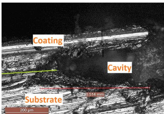
FIGURE 6.48: Coating 1, Corrosion underneath the coating
