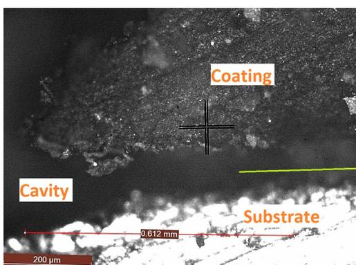
FIGURE 6.50: Coating 3, Corrosion underneath the coating
