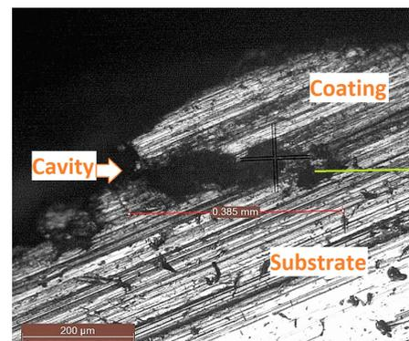
FIGURE 6.49: Coating 2, Corrosion underneath the coating
