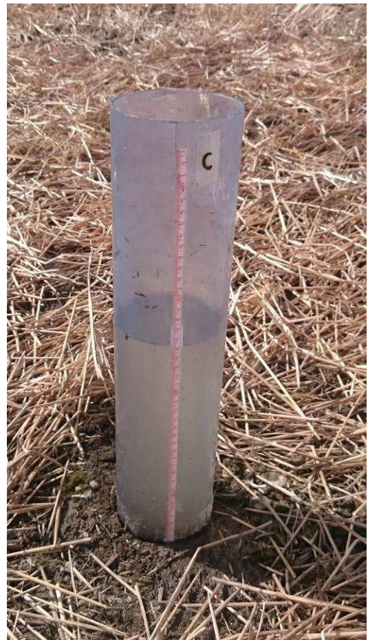
Figure 4: Infiltrometer tube used at infiltration test at Overvik.
