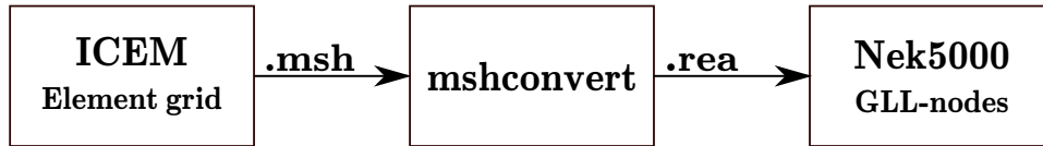
FIGURE 4.1: Visualization of how the mesh is created. The elemental mesh is first generated using ICEM, the script mshconvert converts this to a .rea-file and finally the distribution of the GLL-nodes is done during the initialization in Nek5000
