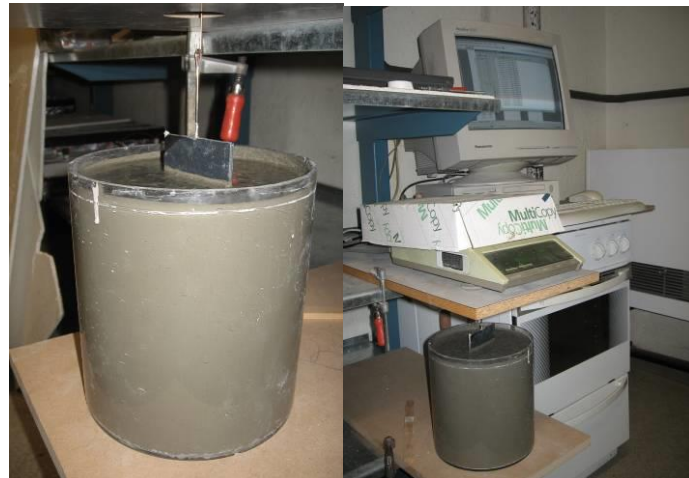
Fig. 6: Test set up for plate test
