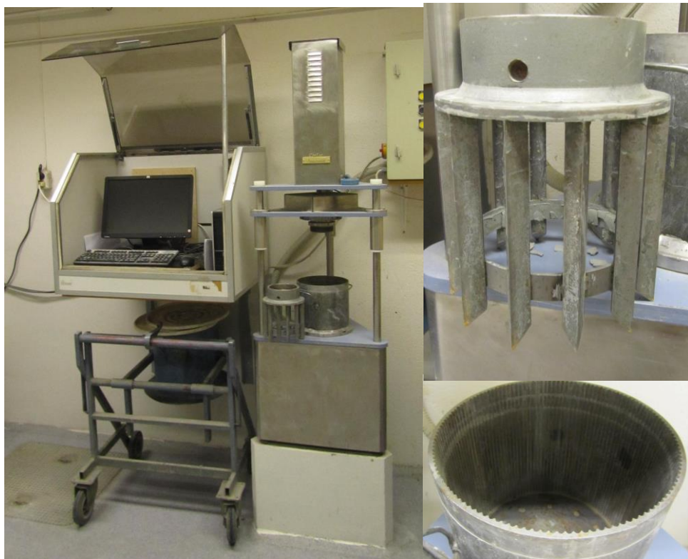
Fig. 4: ConTec4 with rotating container and static core
