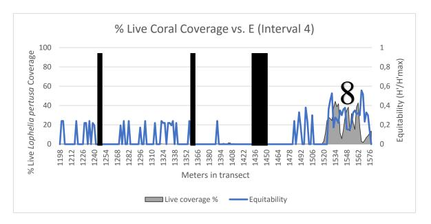
Figure 29: Fourth interval of a total of four intervals on the Tautra sill transect. Percent live L. pertusa coverage is indicated with the left, primary y-axis. The secondary y-axis to the right indicates Shannon's diversity index, H'. Meter travel distance done by the ROV is indicated with the x-axis. Black bars represent points with no data.
