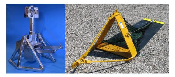
Figure 4: On the left is a box corer, this particular boxcorer is from the manufacturer KC Denmark A/S. It has a typical design for the type of bottom substrate sampling gear. On the right is a triangular bottom dredge also from the manufacturer KC Denmark A/S. The sledge also has a typical design with a triangular metal fram to scrape benthic fauna from the seabed. (KC Denmark A/S, 2016b, KC Denmark A/S, 2016a)
