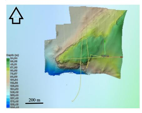
Figure 6: Digital terrain model of the survey area and transect lines from the Beitstadfjord survey. The arrow in the upper left corner indicates north direction. Black line in the lower left corner has a scale of 200 m. Dark green indicates depth of approximately 25 m, dark blue indicates 200 m depth or more. The area is within the red circle in Figure 5.
