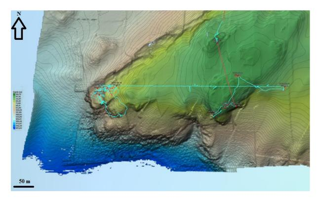
Figure 10: Digital terrain model from survey done at Hoøyskjæret in Beitstadfjord 19<sup>th</sup> of May 2015. Red and blue line indicates transect of the ROV. Red colour = no video coverage, blue = video coverage. Line in lower left corner indicates 50 m distance. Dark green is approximately 35 m depth, dark blue and light blue is 200 m depth or more. Contour lines indicates 2 m interval change in depth. Upper left arrow indicates northwards direction.
