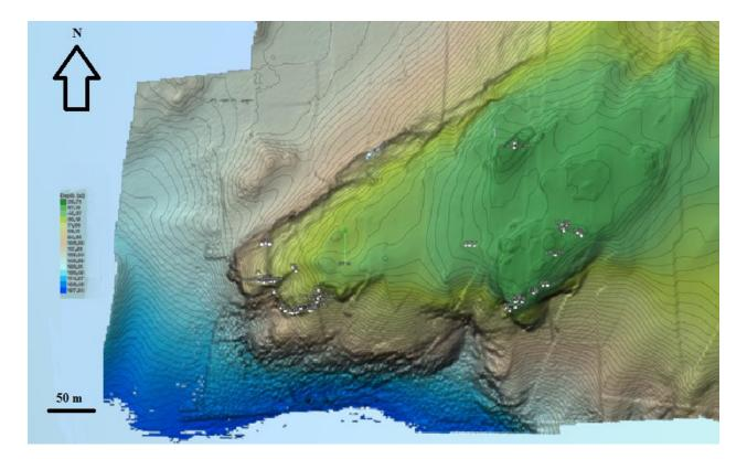
Figure 11: Digital terrain model from Hoøyskjæret. White dots in figure indicates location of corals registered from video survey. Line in lower left corner indicates 50 m length. Dark green indicates approximately 35 m depth, dark blue indicates 200 m depth or more. Contour lines indicates 2 m change in depth. Upper left arrow indicates northward direction.
