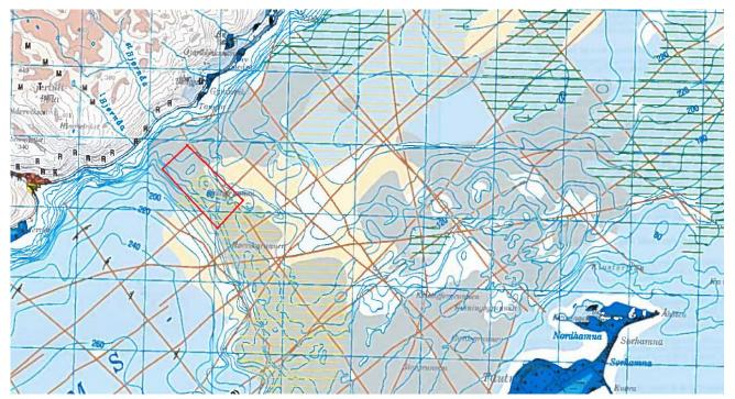
Figure 1: Geological map over the Tautra ridge provided by NGU. Scale 1:50 000. The red box indicates the area surveyed during the cruises 25th and 26th of June 2015. The colours within the box indicates a seafloor covered in till deposits in a relatively thin layer (grey/green colour) and glaciofluvial deposits (light yellow). White areas indicates bedrock. Source: (Reite and Olsen, 2002).
