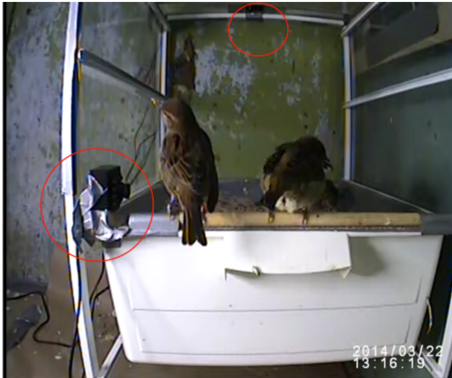
Figure 3. The feeder used in the social context assays. This is a screenshot from a video obtained with the camera that is pointing directly at the entrance of the feeder. The two other cameras used in the video analysis are visible here; one to the left of the entrance, pointing along the entrance perch, and one just visible at the top, pointing down on the feeder through a hole in the ceiling. Note that all sides except the entrance were covered with plexiglass. Size of the feeder: 60 cm x 50 cm. The floor of the feeder was raised up almost to the entrance perch.
