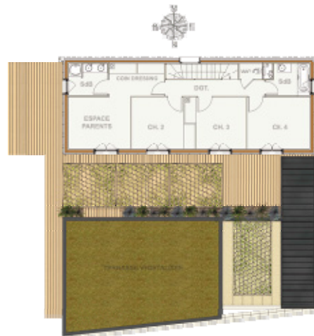
First floor. The roof of the garage is covered with vegetation to improve temperature during the summer.
