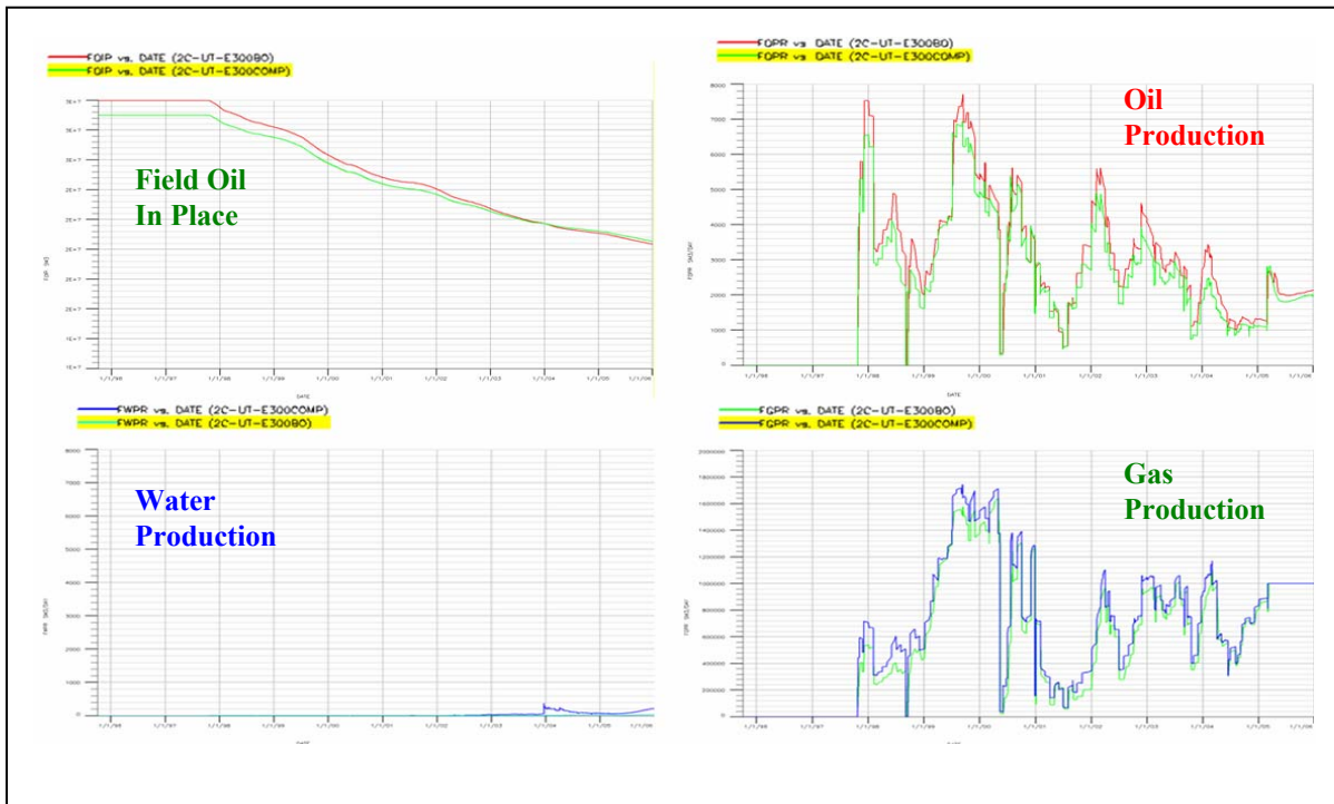
Figure 48: The Comparison Simulation Result (for H and I Segment) between Eclipse 300 Compositional and Eclipse 300 Black Oil
