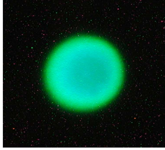
Fig. 7. Intensity profile of the TH radiation from the 4.5 \mu\text{m} core of SF6 PCF, taken at approximately 3 cm free propagation distance after the fiber end. The individual mode patterns can not be resolved.
