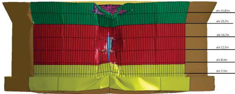
Figure 8.11 Cracks on the Platform_Head on_4m/s
